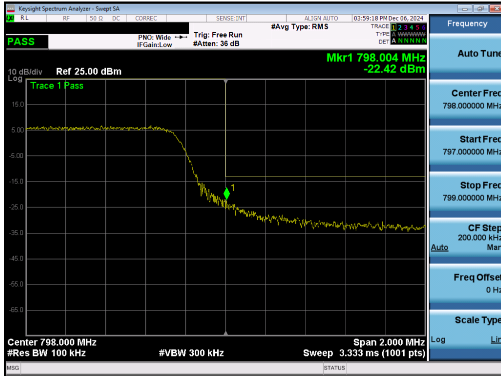
Plot 7-123. Upper Band Edge Plot (LTE Band 14, 5MHz QPSK - RB Size 25 – Ant2)
