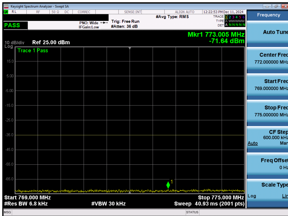
Plot 7-110. Lower Emission Mask Plot (LTE Band 14, 5MHz QPSK - RB Size 25 – Ant5)
