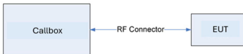
Figure 7-1. Test Instrument & Measurement Setup
