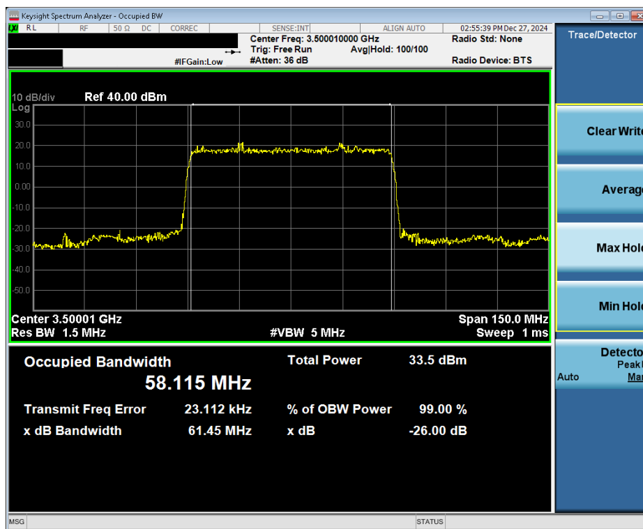
Plot 7-14. Occupied Bandwidth Plot (NR Band n77 DoD - 60MHz \pi/2 BPSK - Full RB - Ant6)
