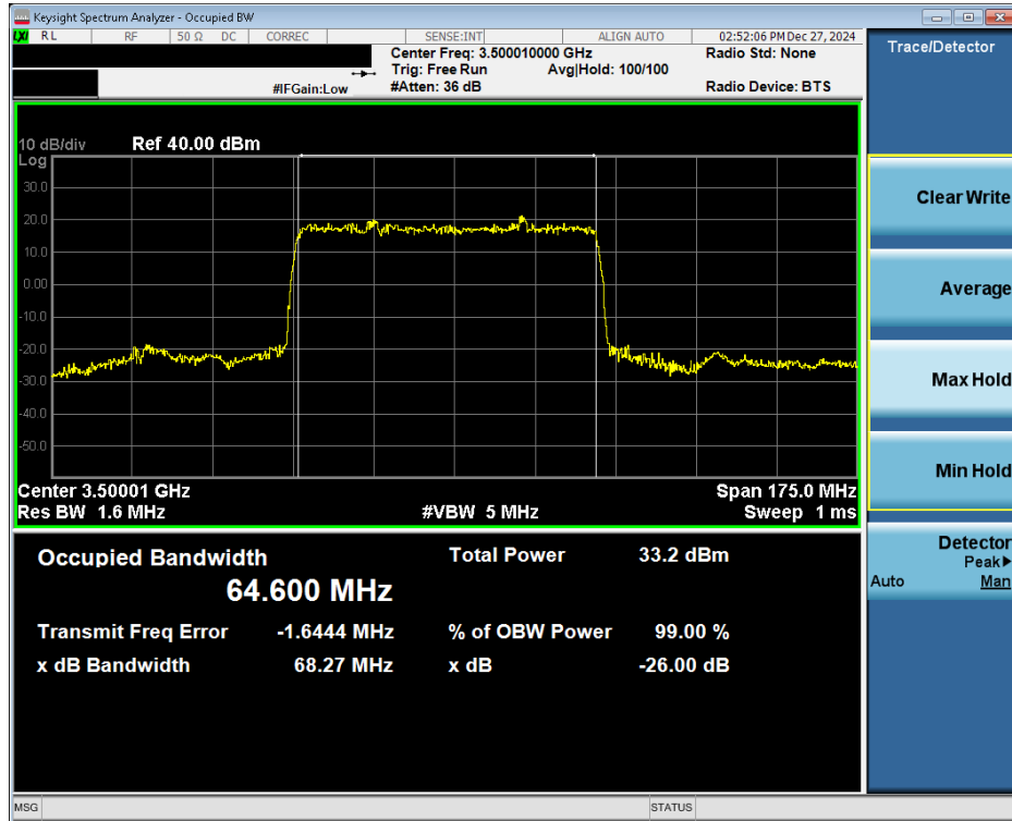
Plot 7-11. Occupied Bandwidth Plot (NR Band n77 DoD - 70MHz \pi/2 BPSK - Full RB - Ant6)
