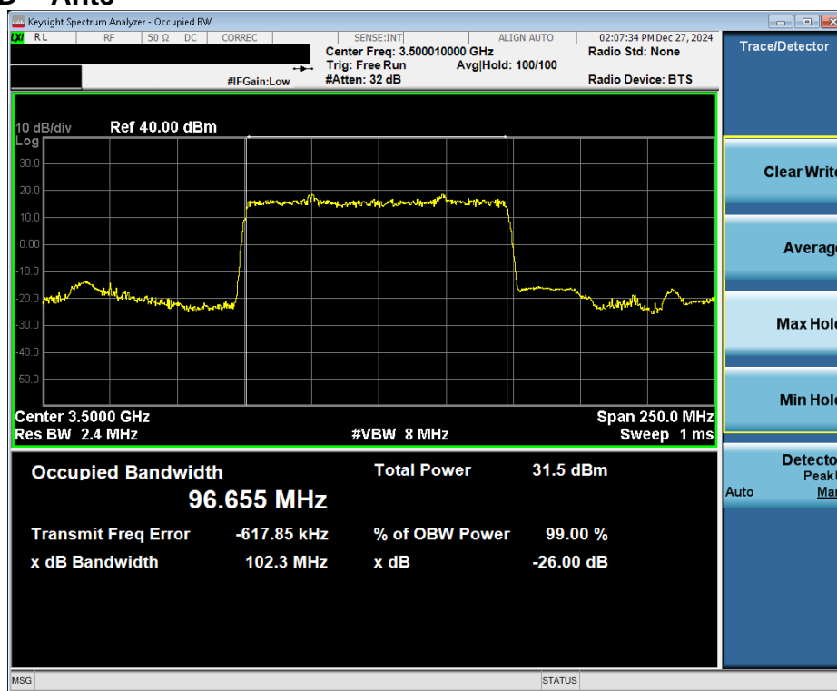
Plot 7-1. Occupied Bandwidth Plot (NR Band n77 DoD - 100MHz \pi/2 BPSK - Full RB - Ant6)
