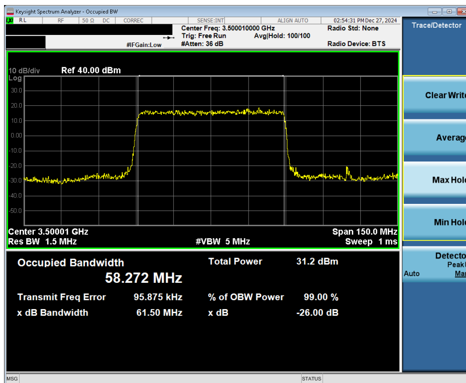
Plot 7-16. Occupied Bandwidth Plot (NR Band n77 DoD - 60MHz 16-QAM - Full RB - Ant6)
