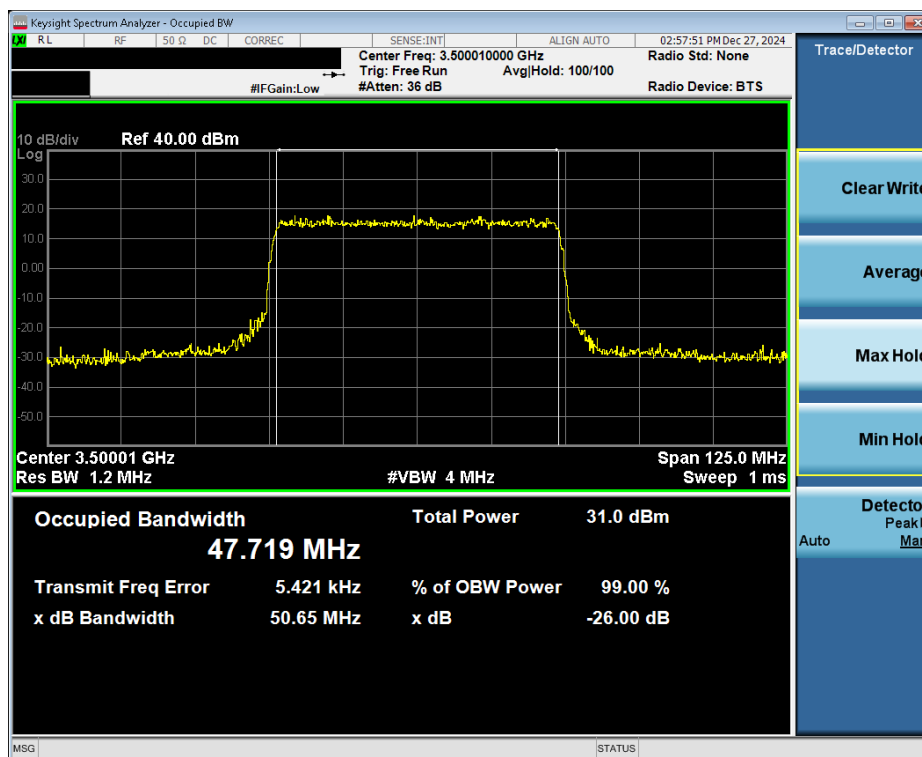
Plot 7-18. Occupied Bandwidth Plot (NR Band n77 DoD - 50MHz QPSK - Full RB - Ant6)
