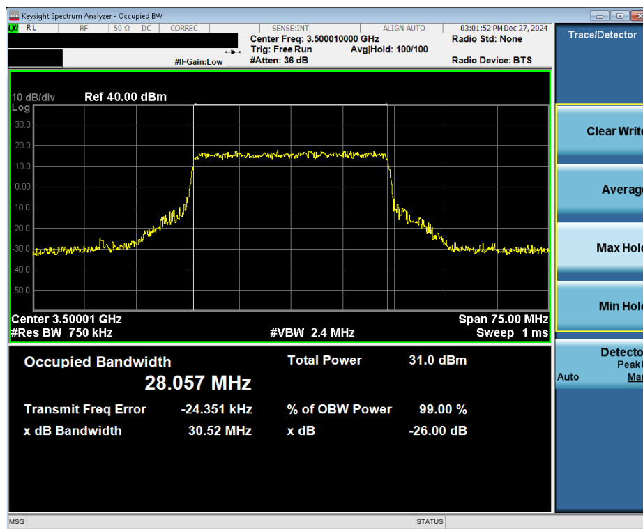
Plot 7-25. Occupied Bandwidth Plot (NR Band n77 DoD - 30MHz 16-QAM - Full RB - Ant6)
