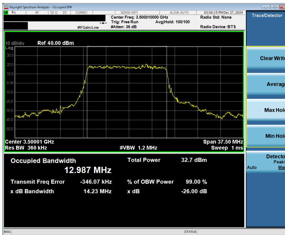
Plot 7-29. Occupied Bandwidth Plot (NR Band n77 DoD - 15MHz \pi/2 BPSK - Full RB - Ant6)
