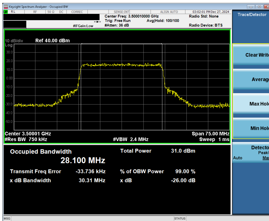
Plot 7-24. Occupied Bandwidth Plot (NR Band n77 DoD - 30MHz QPSK - Full RB - Ant6)
