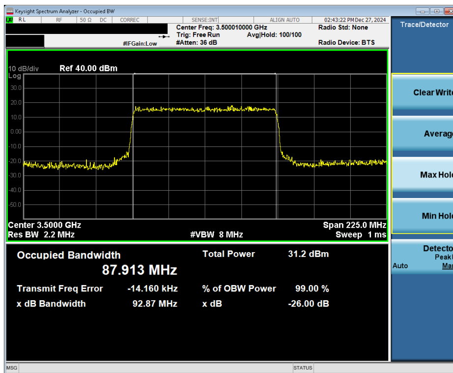
Plot 7-7. Occupied Bandwidth Plot (NR Band n77 DoD - 90MHz 16-QAM - Full RB - Ant6)
