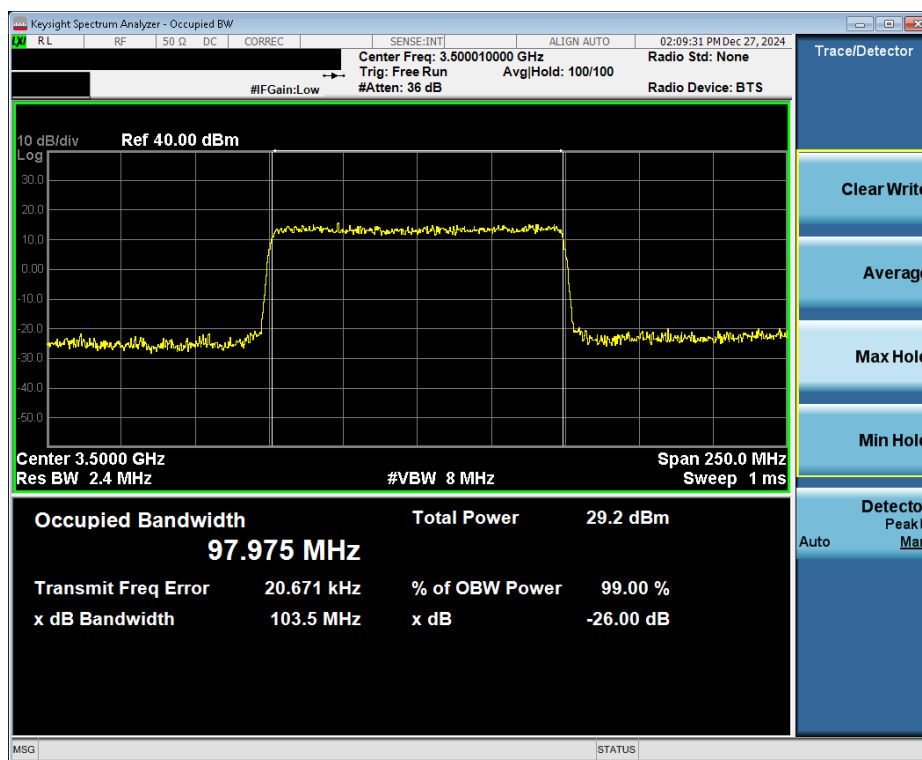
Plot 7-2. Occupied Bandwidth Plot (NR Band n77 DoD - 100MHz QPSK - Full RB - Ant6)
