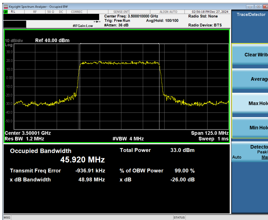
Plot 7-17. Occupied Bandwidth Plot (NR Band n77 DoD - 50MHz \pi/2 BPSK - Full RB - Ant6)
