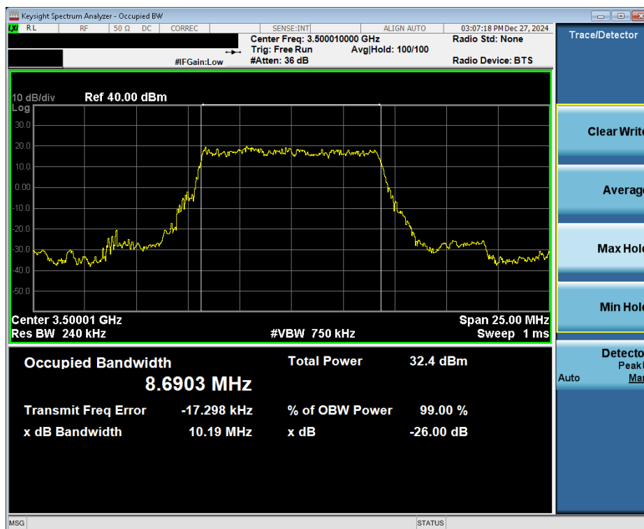
Plot 7-32. Occupied Bandwidth Plot (NR Band n77 DoD - 10MHz \pi/2 BPSK - Full RB - Ant6)
