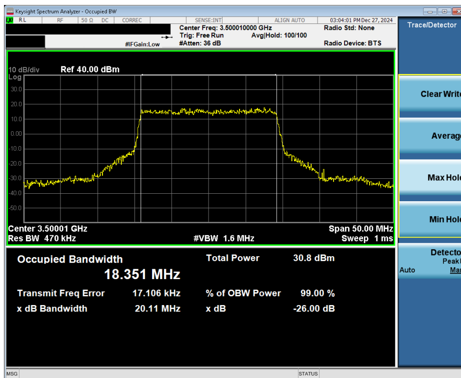
Plot 7-28. Occupied Bandwidth Plot (NR Band n77 DoD - 20MHz 16-QAM - Full RB - Ant6)
