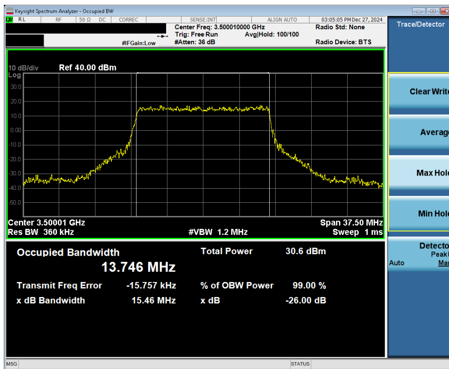
Plot 7-31. Occupied Bandwidth Plot (NR Band n77 DoD - 15MHz 16-QAM - Full RB - Ant6)
