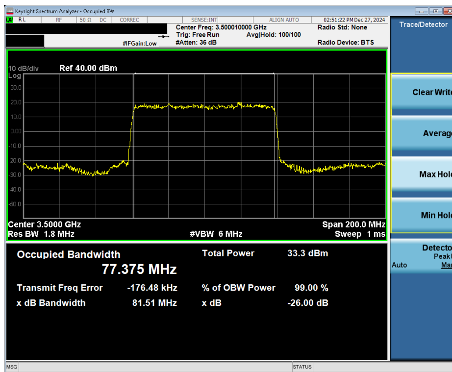
Plot 7-8. Occupied Bandwidth Plot (NR Band n77 DoD - 80MHz \pi/2 BPSK - Full RB - Ant6)
