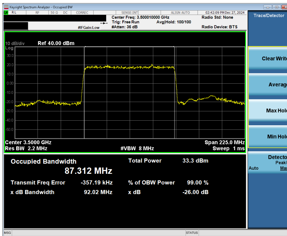
Plot 7-5. Occupied Bandwidth Plot (NR Band n77 DoD - 90MHz \pi/2 BPSK - Full RB - Ant6)
