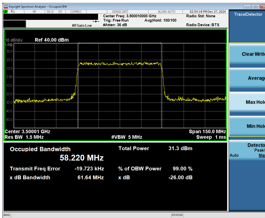
Plot 7-15. Occupied Bandwidth Plot (NR Band n77 DoD - 60MHz QPSK - Full RB - Ant6)
