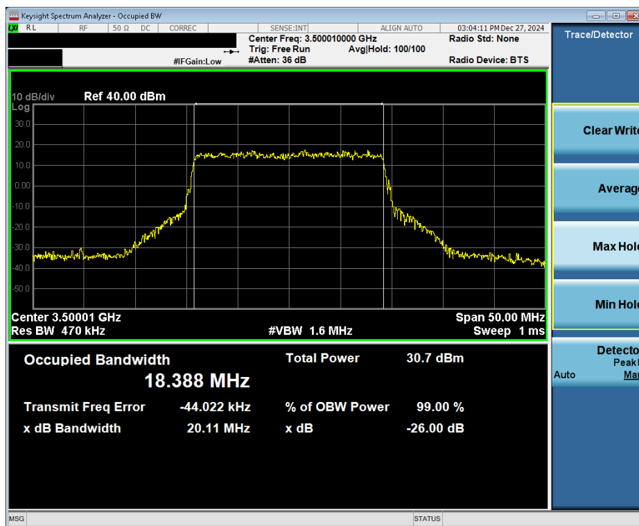
Plot 7-27. Occupied Bandwidth Plot (NR Band n77 DoD - 20MHz QPSK - Full RB - Ant6)
