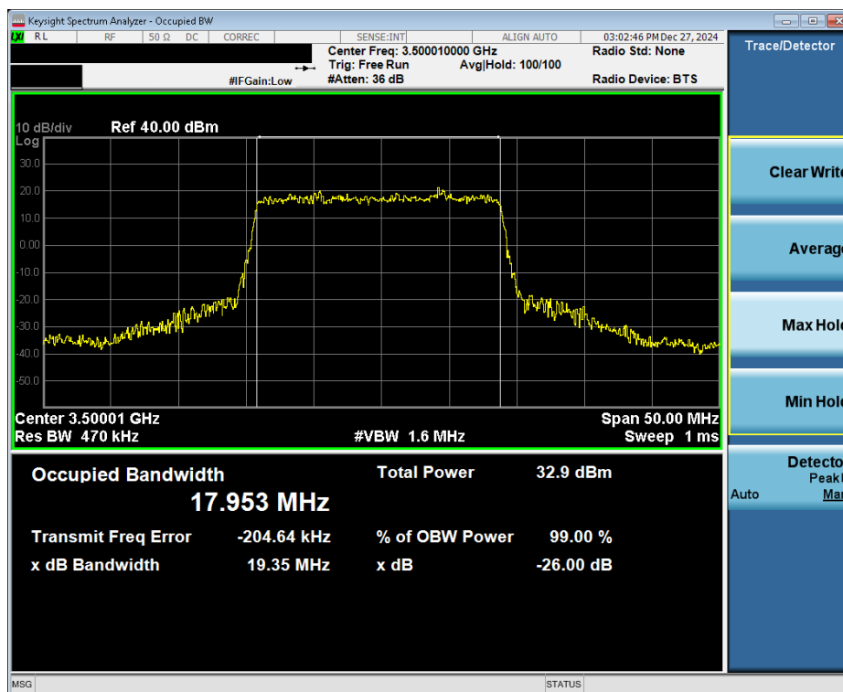
Plot 7-26. Occupied Bandwidth Plot (NR Band n77 DoD - 20MHz \pi/2 BPSK - Full RB - Ant6)
