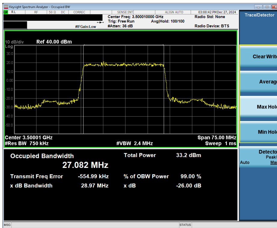
Plot 7-23. Occupied Bandwidth Plot (NR Band n77 DoD - 30MHz \pi/2 BPSK - Full RB - Ant6)
