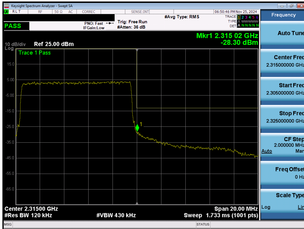
Plot 7-157. Upper Band Edge Plot (LTE Band 30 - 10MHz QPSK – Full RB - Ant1)
