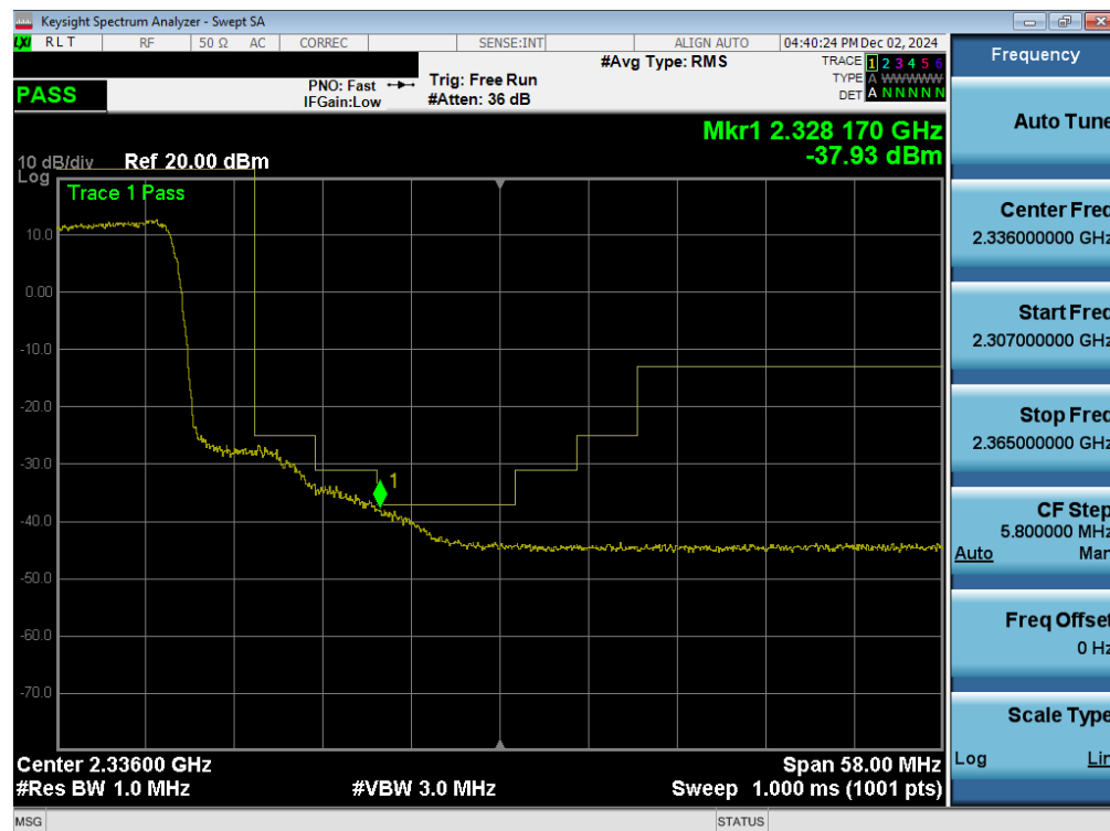
Plot 7-158. Extended Upper Band Edge Plot (LTE Band 30 A-MPR - 10MHz QPSK – Full RB - Ant1)
