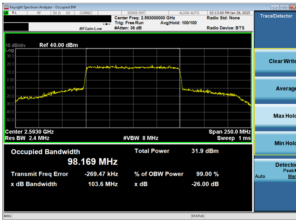
Plot 7-111. Occupied Bandwidth Plot (NR Band n41 - 100MHz 16-QAM - Full RB - Ant1)
