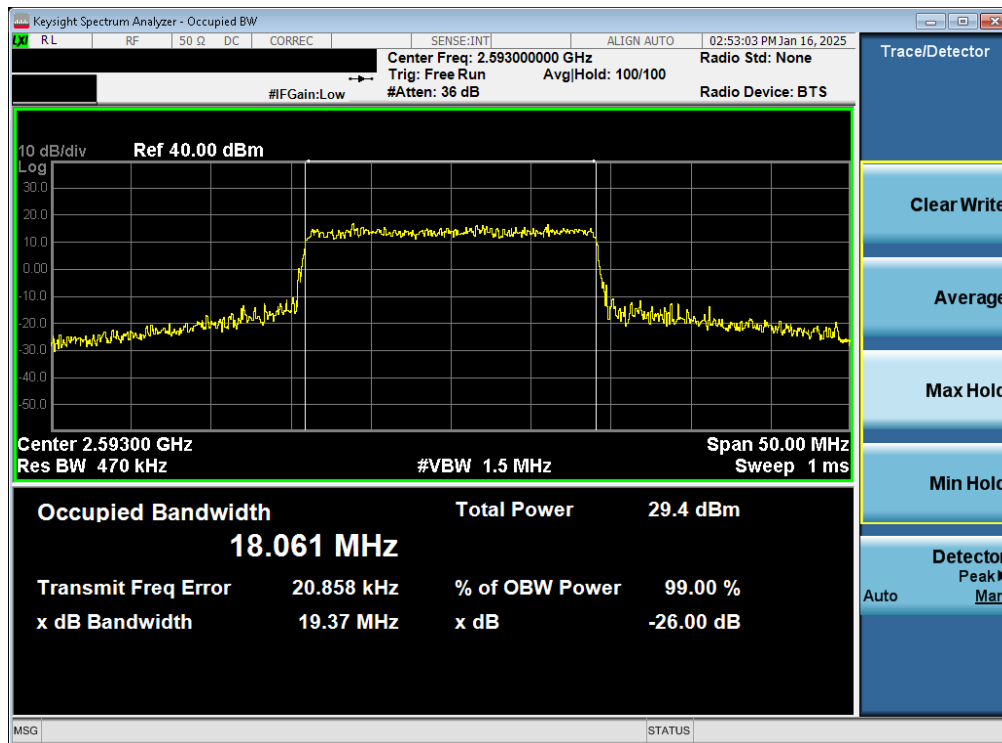
Plot 7-69. Occupied Bandwidth Plot (LTE Band 41(PC3)/38 - 20MHz 16-QAM - Full RB - Ant6)
