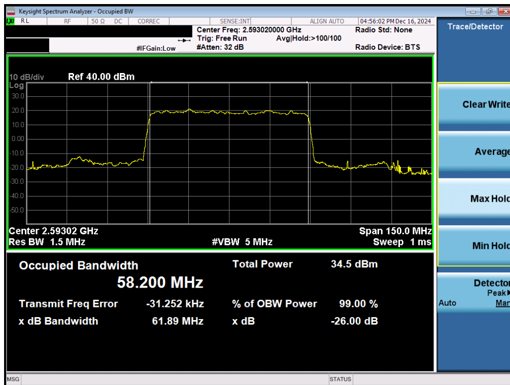
Plot 7-39. Occupied Bandwidth Plot (NR Band n41 - 60MHz \pi/2 BPSK - Full RB - Ant1)
