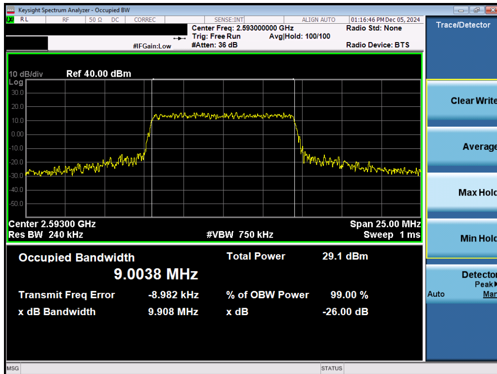
Plot 7-18. Occupied Bandwidth Plot (LTE Band 41(PC3)/38 - 10MHz 16-QAM - Full RB - Ant1)
