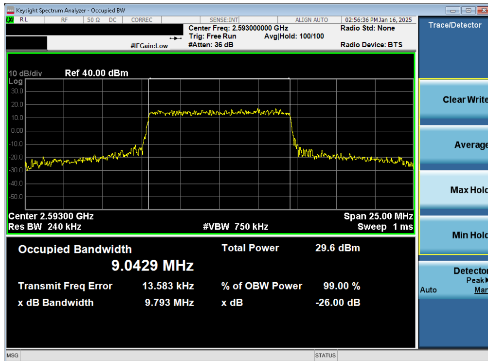
Plot 7-73. Occupied Bandwidth Plot (LTE Band 41(PC3)/38 - 10MHz 16-QAM - Full RB - Ant6)
