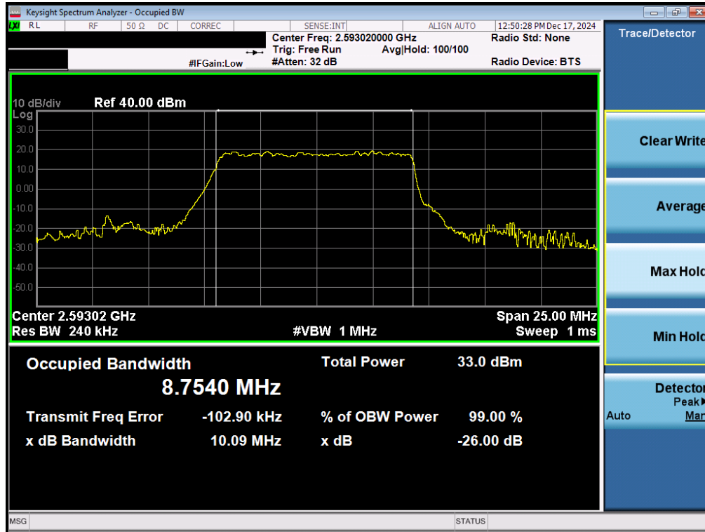
Plot 7-57. Occupied Bandwidth Plot (NR Band n41 - 10MHz \pi/2 BPSK - Full RB - Ant1)
