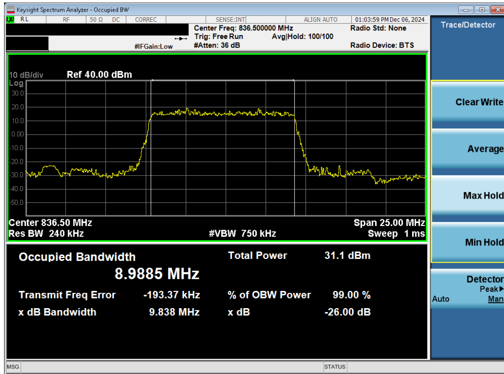
Plot 7-18. Occupied Bandwidth Plot (NR Band n5 - 10MHz \pi/2 BPSK - Full RB - Ant 5)
