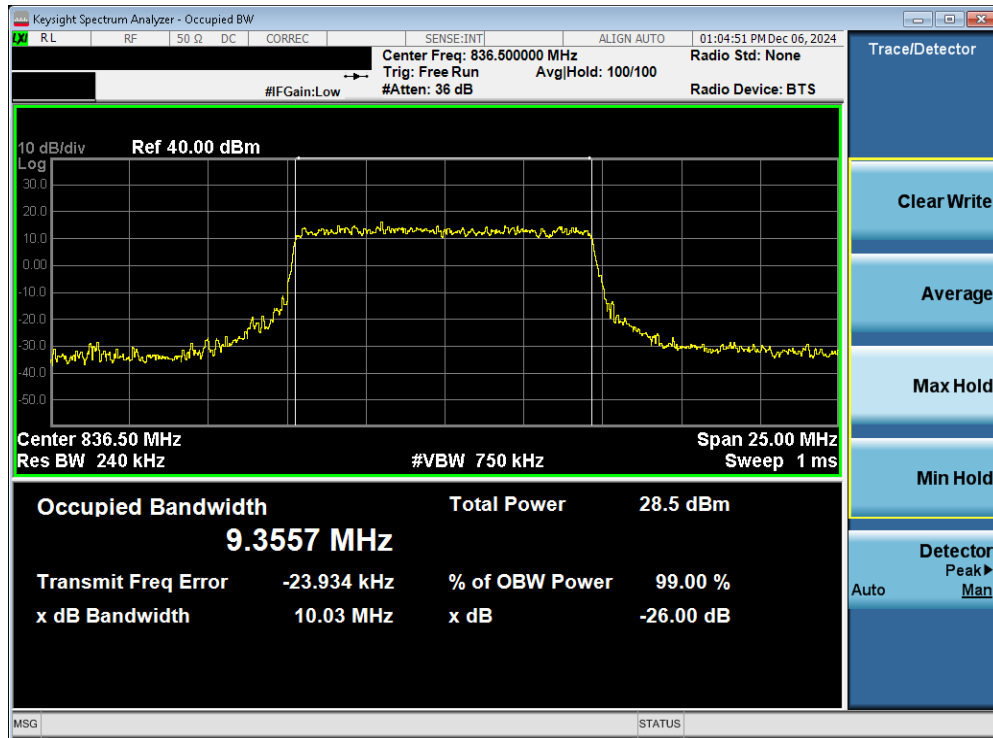
Plot 7-20. Occupied Bandwidth Plot (NR Band n5 - 10MHz 16-QAM - Full RB - Ant 5)
