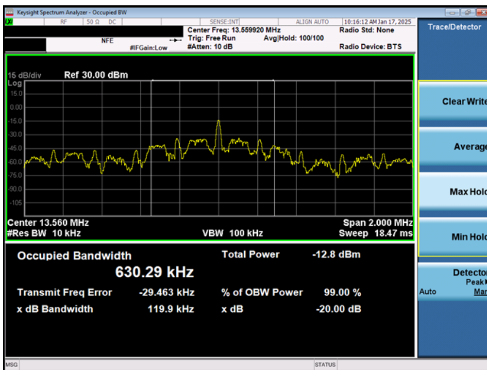
Figure 7-2. Occupied Bandwidth Plot
