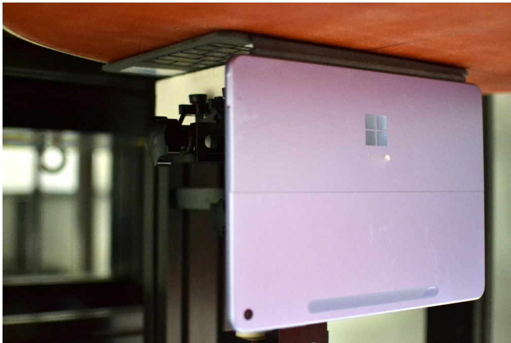
SAR Test Setup Photo 2 – NFC Body, Bottom Edge at 0mm
