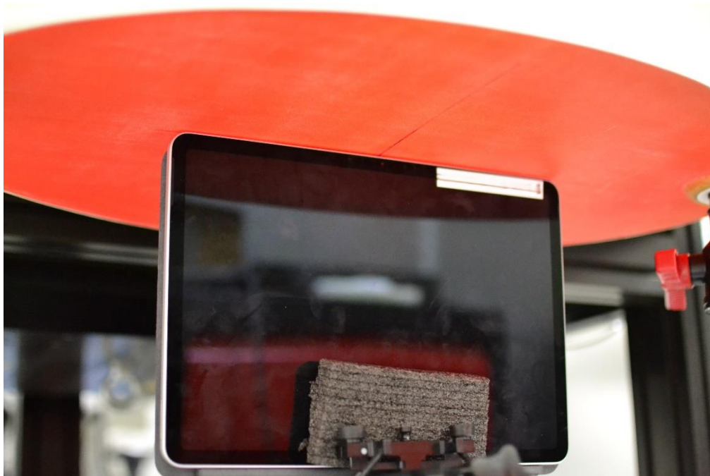
SAR Test Setup Photo 4 – NFC Body with Keyboard, Top Edge at 0mm
