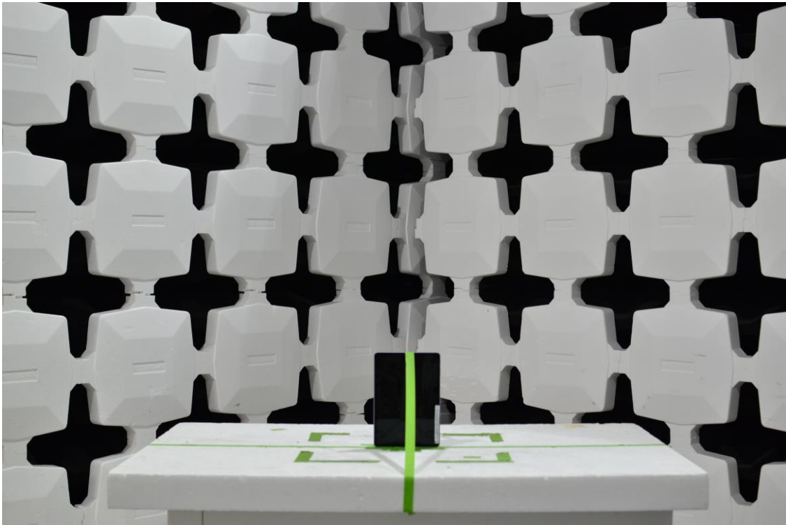
Figure 3. Test Setup – Y Position – 30MHz-1GHz – NFC
