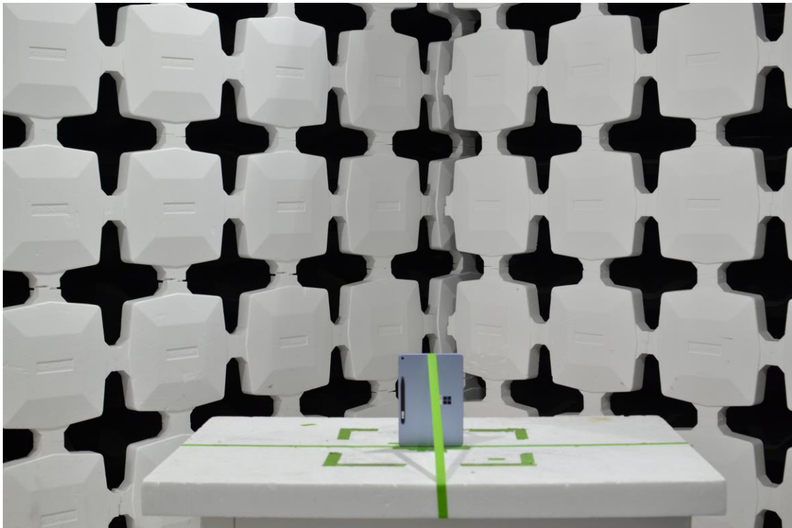
Figure 8. Test Setup – Y Position – 30MHz-1GHz – Pen Charging
