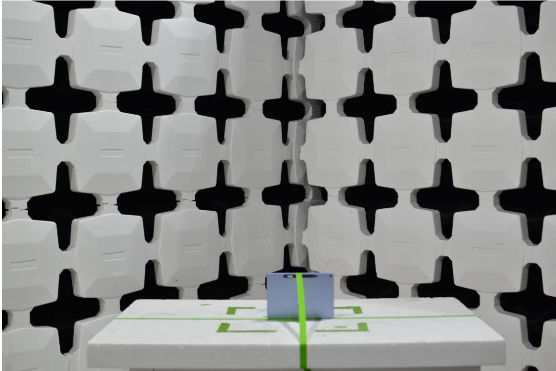
Figure 9. Test Setup – Z Position – 30MHz-1GHz – Pen Charging
