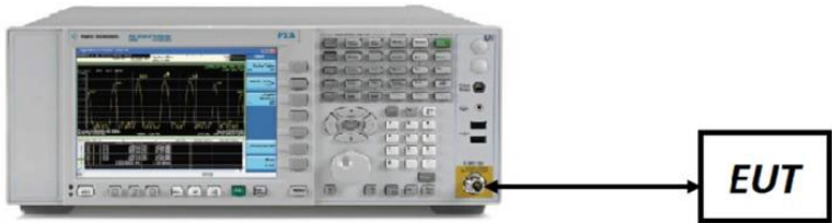
Figure 7-4. Conducted Test Setup > 1GHz
