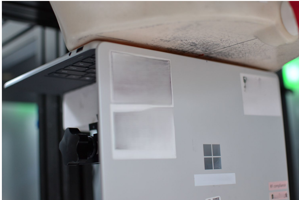
Test Setup Photo 4 – Body, Bottom Edge at 0mm, Antenna R and L
