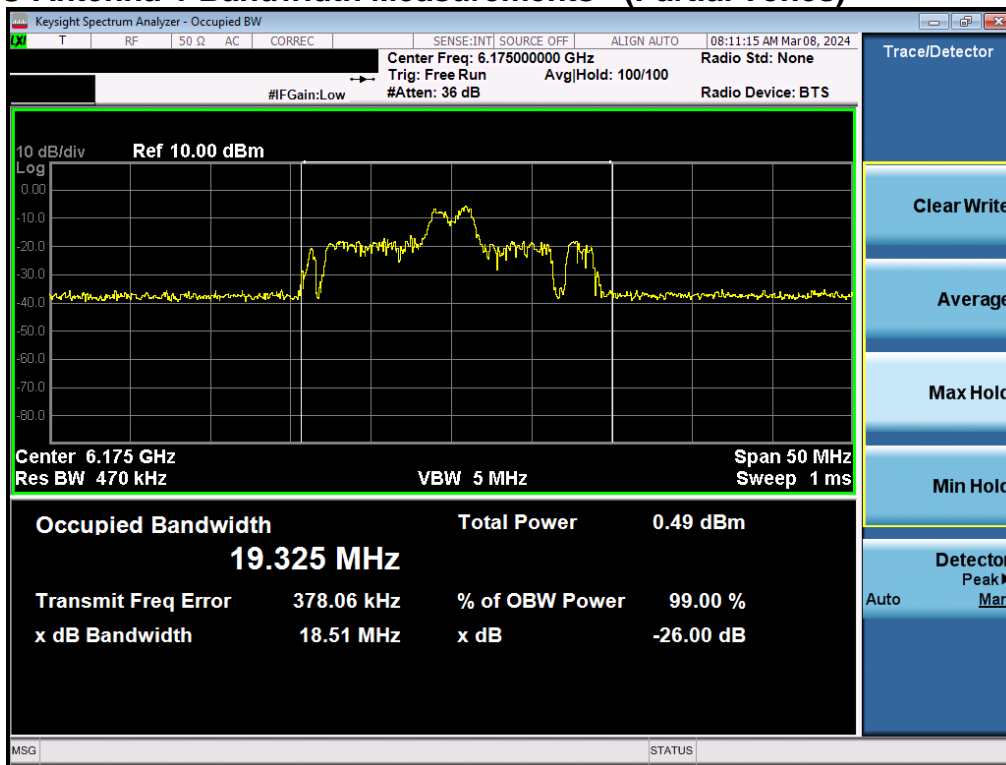
Plot 7-1. Occupied Bandwidth Plot MIMO ANT1 (20MHz BW 802.11be (26 Tones) (UNII Band 5) – Ch. 45)
