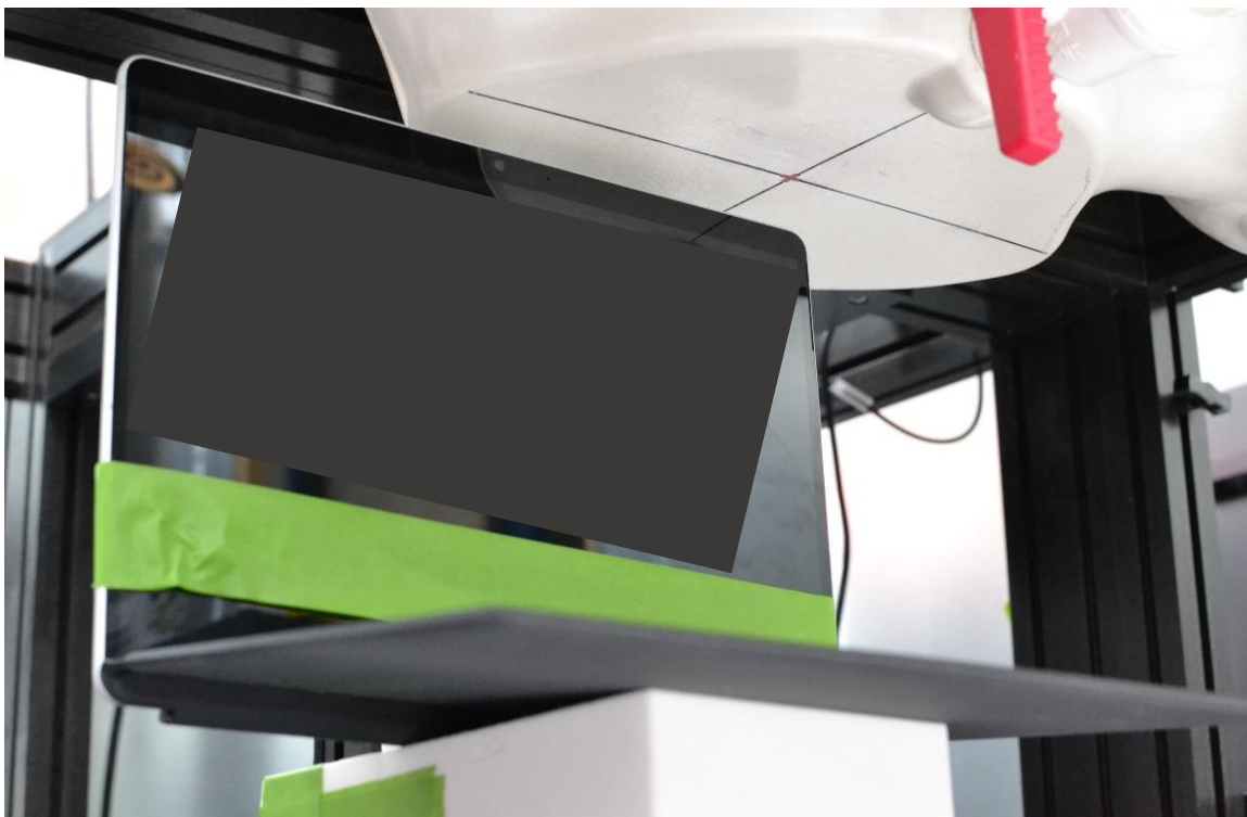
SAR Test Setup Photo 23 – Laptop, Top Edge at 25mm – Antenna 7 & 8
