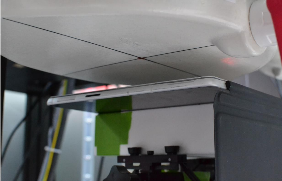
SAR Test Setup Photo 11 – Laptop, Back Side at 25mm – Antenna 7
