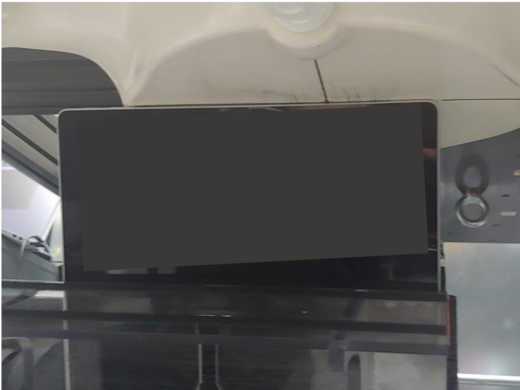
SAR Test Setup Photo 26 – Tablet, Bottom Edge at 0mm – Antenna 3 & 4
