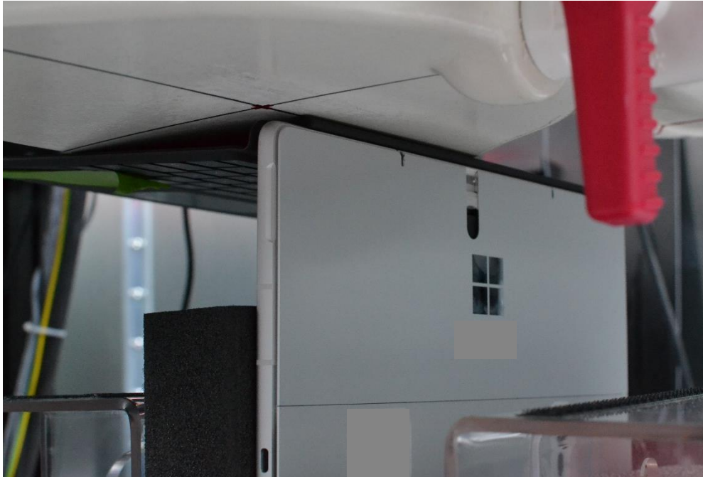
SAR Test Setup Photo 29 – Laptop, Bottom Edge at 0mm – Antenna 5 & 6
