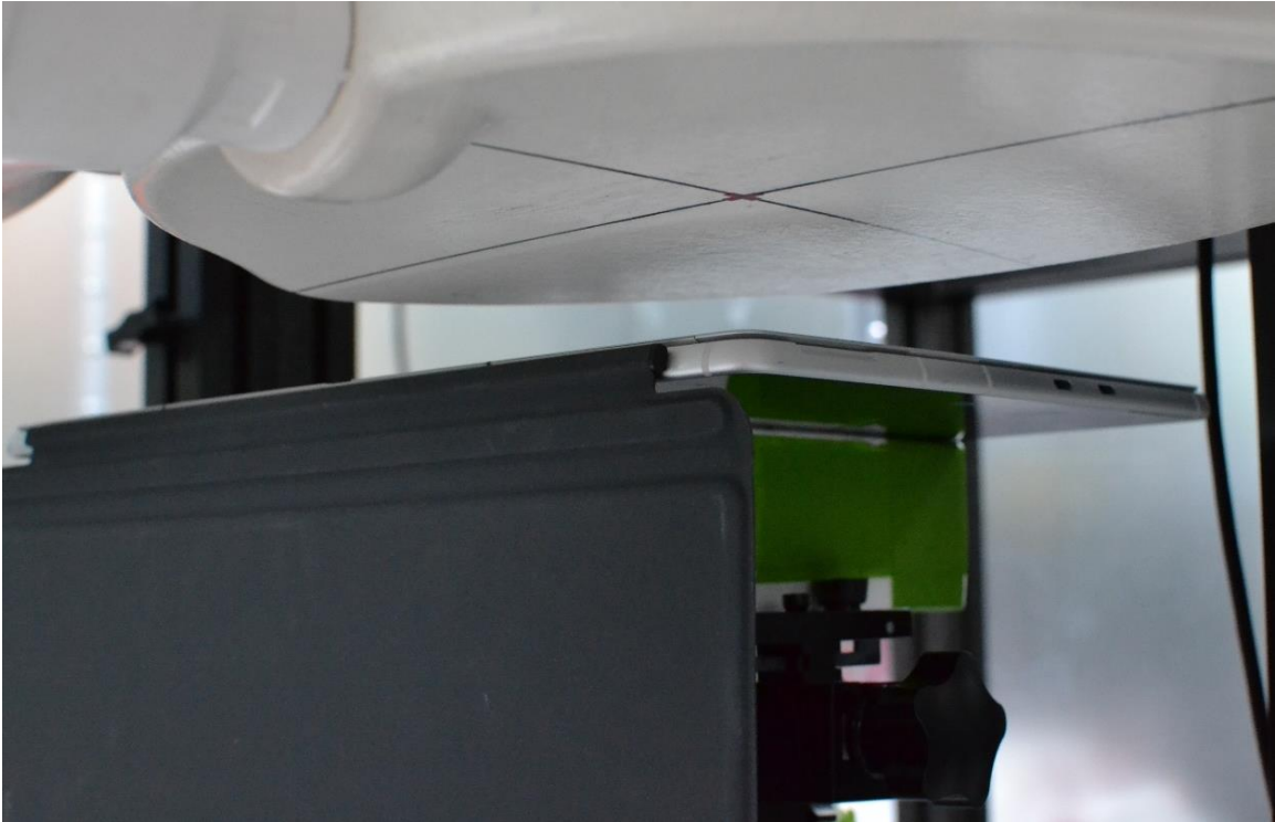
SAR Test Setup Photo 7 – Laptop, Back Side at 25mm – Antenna 5
