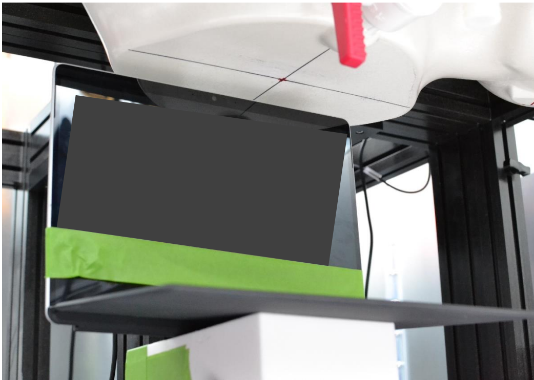
SAR Test Setup Photo 16 – Laptop, Top Edge at 25 mm – Antenna 1 & 2
