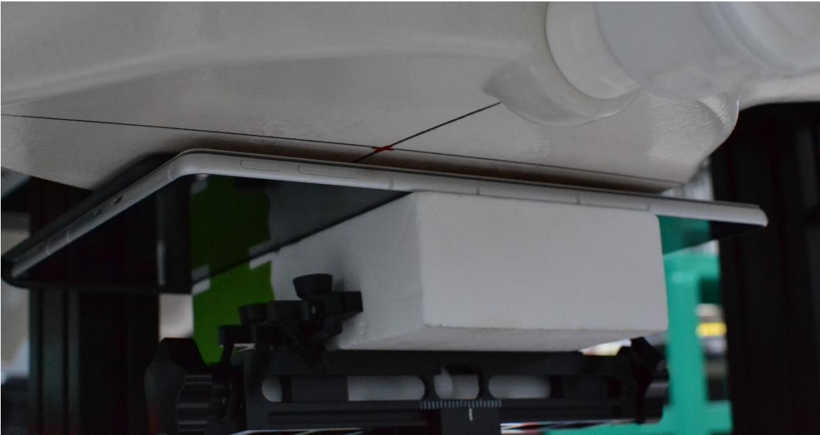
SAR Test Setup Photo 4 – Tablet with keyboard accessory, Back Side at 0mm – Antenna 3 & 4
