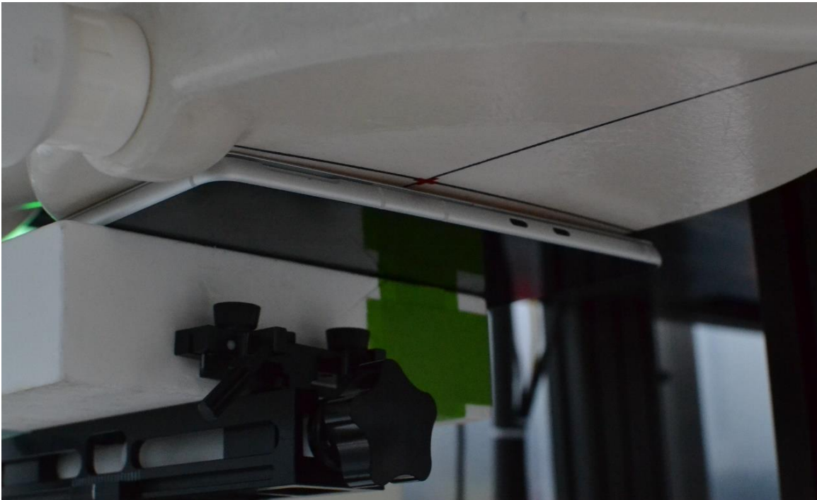
SAR Test Setup Photo 8 – Tablet, Back Side at 0mm – Antenna 6
