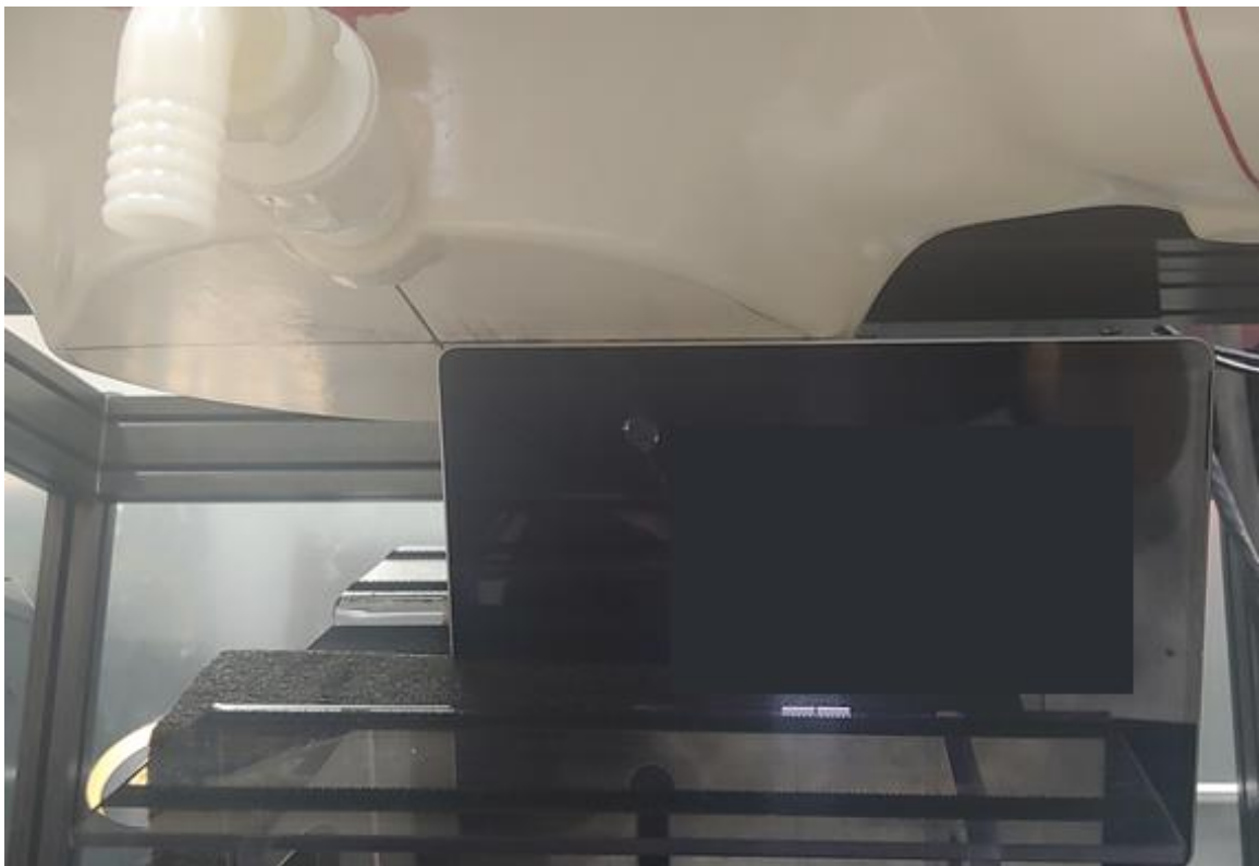
SAR Test Setup Photo 20 – Tablet, Top Edge at 0mm – Antenna 5 & 6
