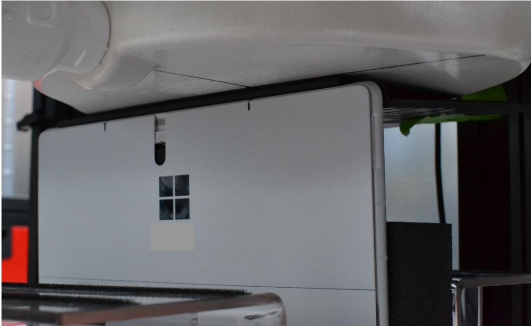
SAR Test Setup Photo 25 – Laptop, Bottom Edge at 0 mm – Antenna 1 & 2
