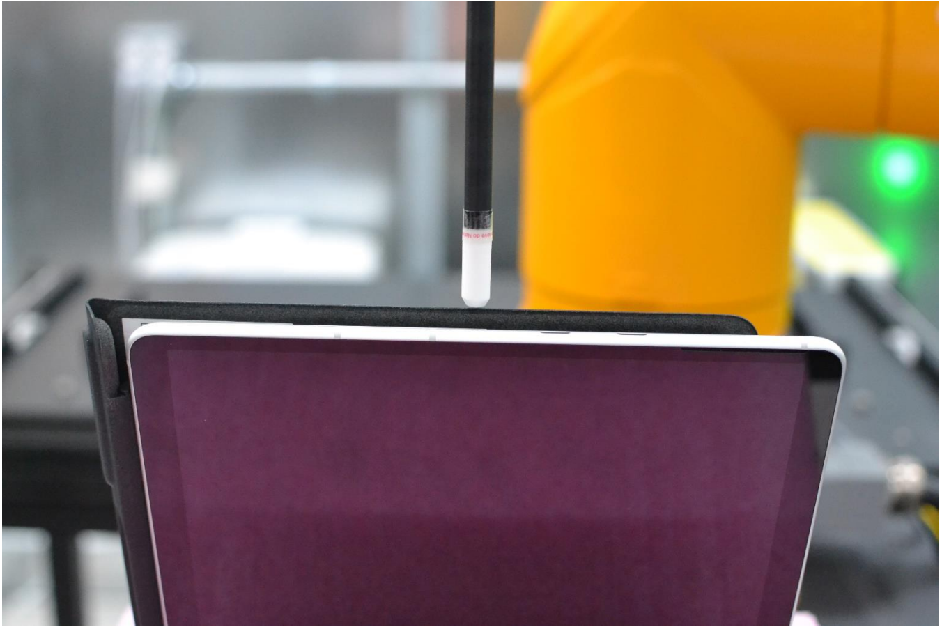
Near Field Power Density Test Setup Photo 45– Left Edge with keyboard accessory at 2 mm
