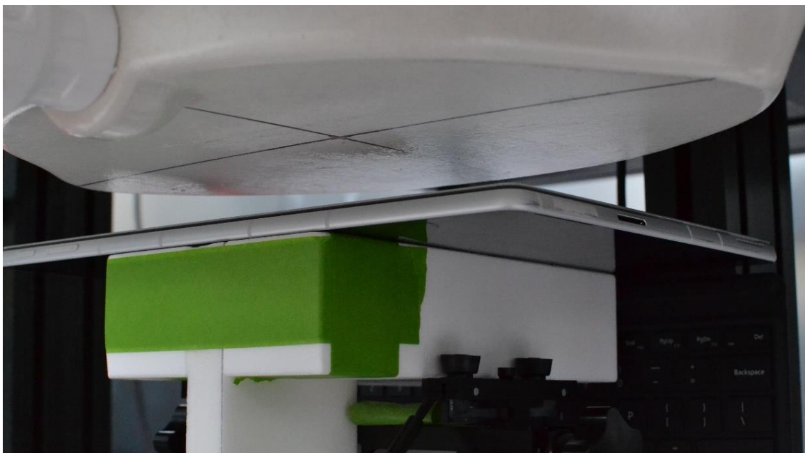
SAR Test Setup Photo 2 – Laptop, Back Side at 25 mm – Antenna 1 & 2
