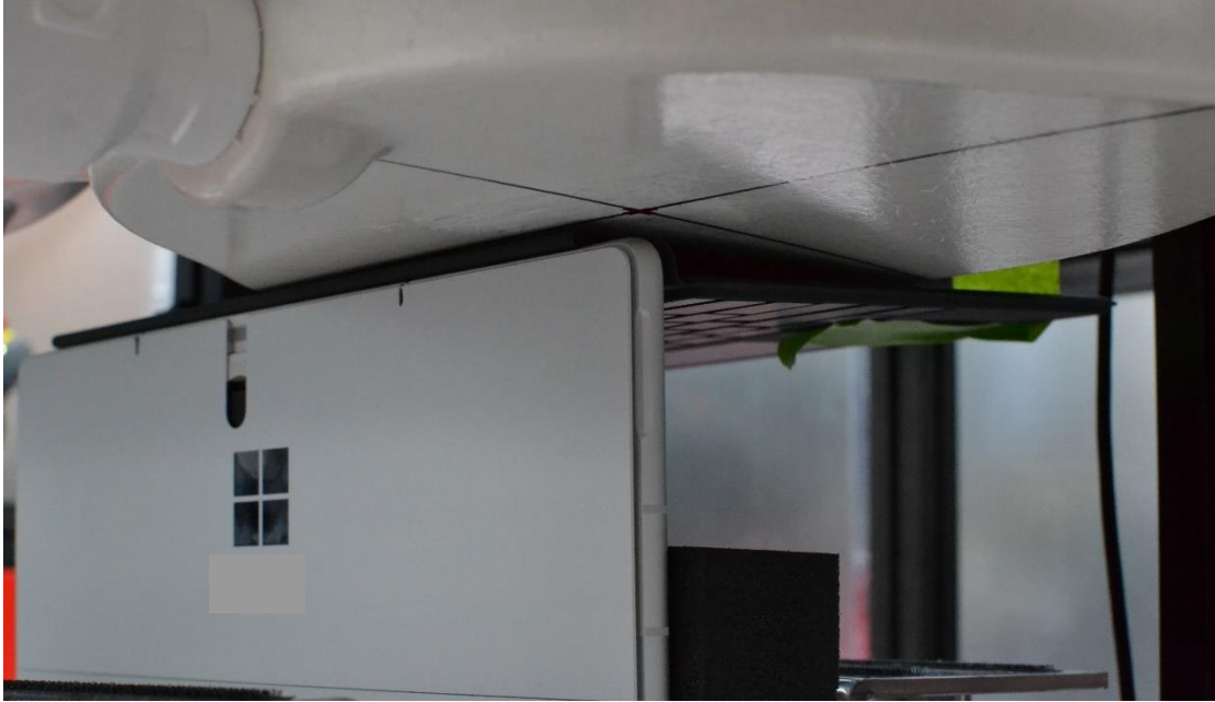
SAR Test Setup Photo 31 – Laptop, Bottom Edge at 0mm – Antenna 7 & 8
