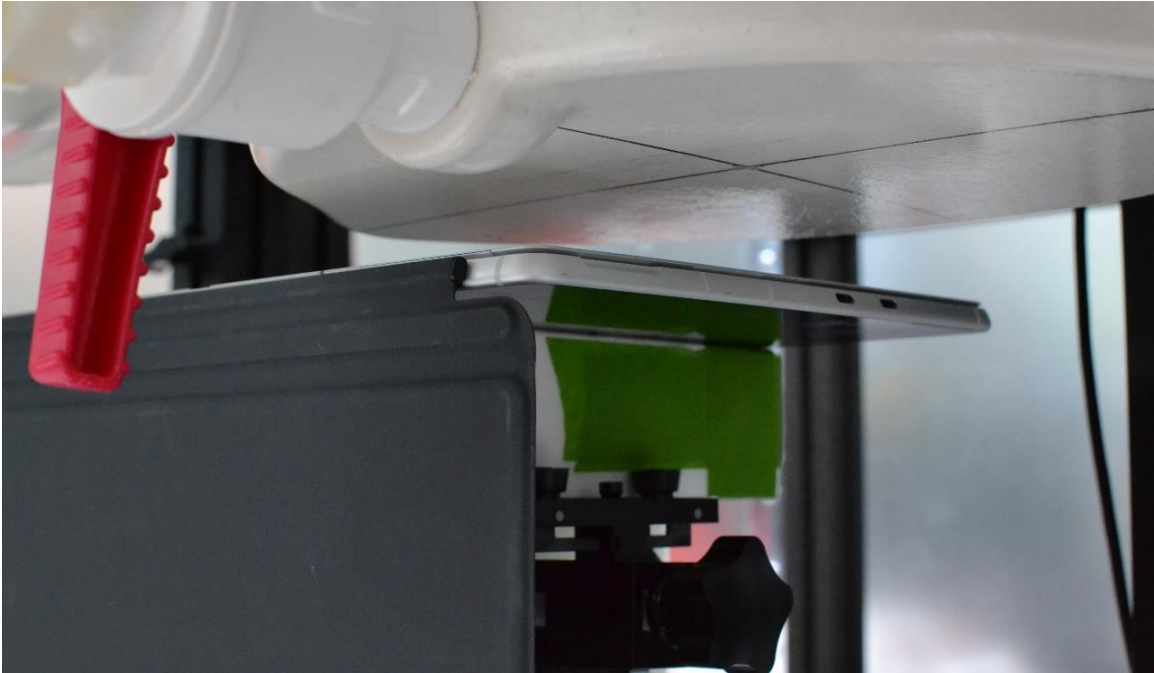
SAR Test Setup Photo 9 – Laptop, Back Side at 25mm – Antenna 6
