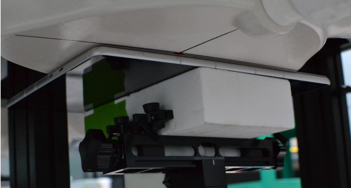
SAR Test Setup Photo 3 – Tablet, Back Side at 0mm – Antenna 3 & 4
