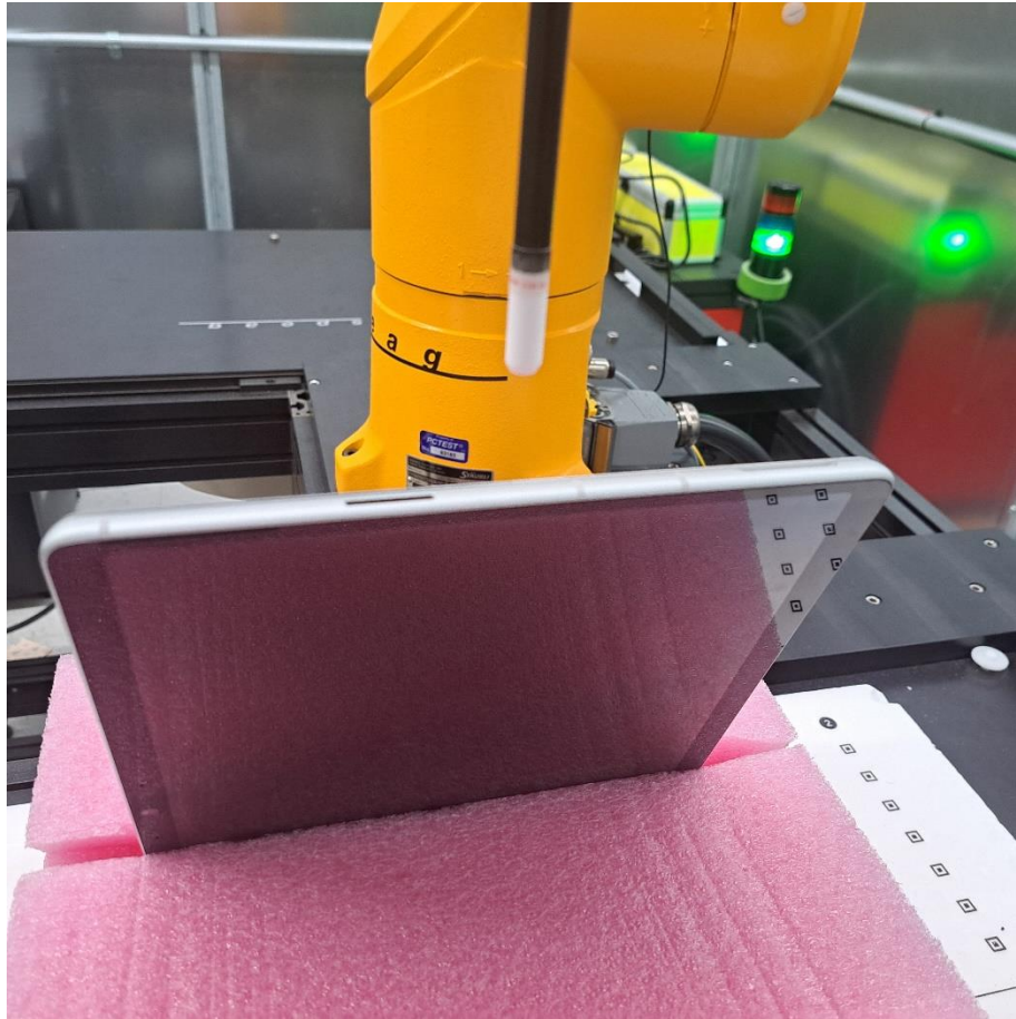
Near Field Power Density Test Setup Photo 43 – Right Edge at 25 mm
