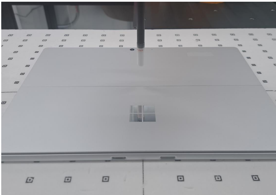
PD Test Setup Photo 39 – Near Field Power Density Back Side at 25 mm
