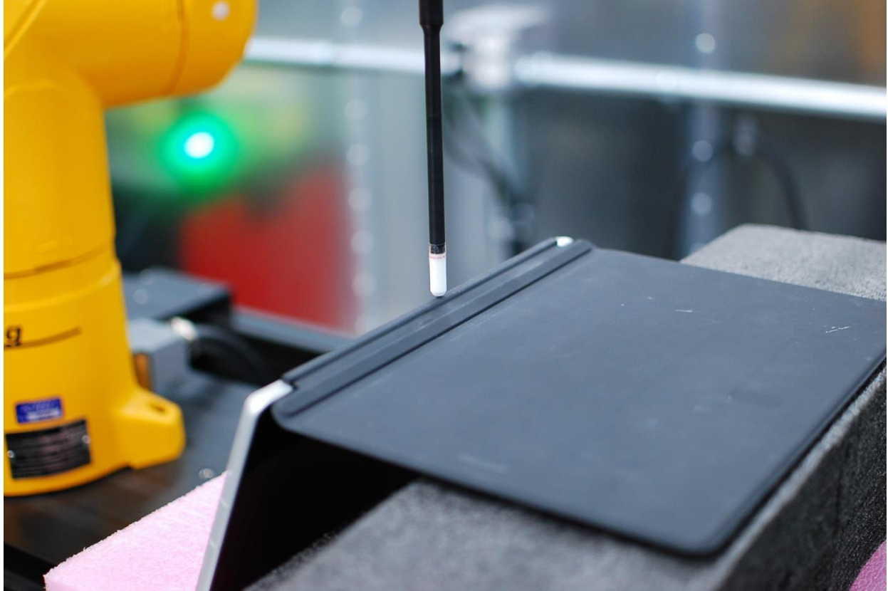
Near Field Power Density Test Setup Photo 48 – Laptop Bottom Edge at 2 mm
