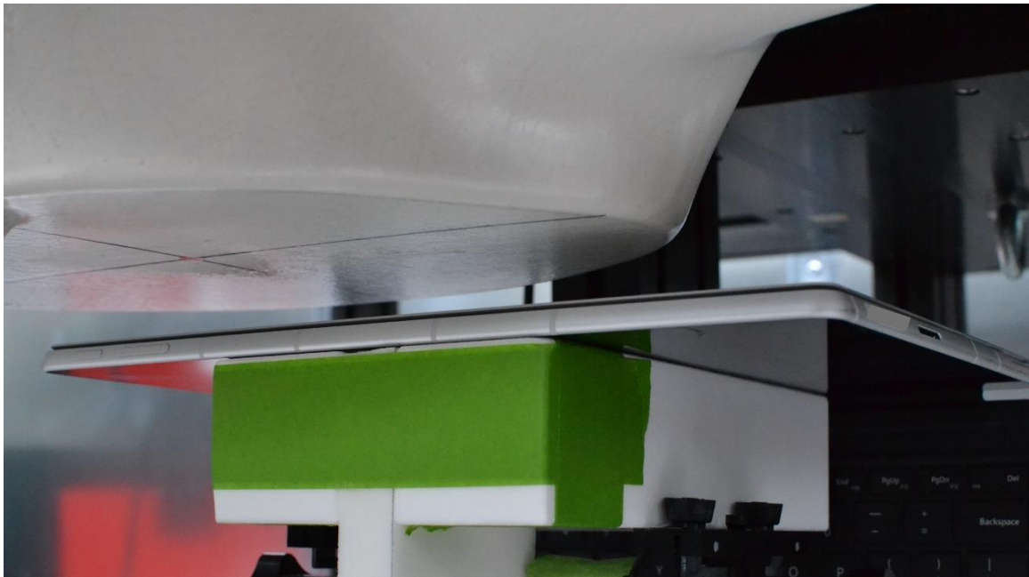
SAR Test Setup Photo 5 – Laptop, Back Side at 25mm – Antenna 3 & 4
