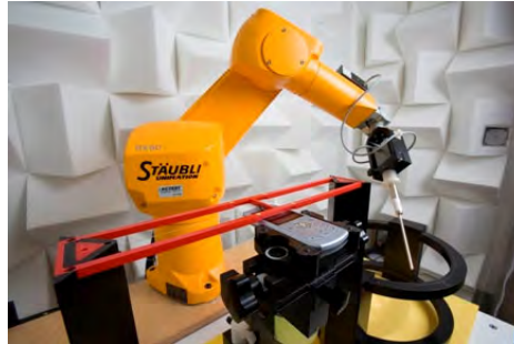
Figure 4-3 SPEAG Robotic System
