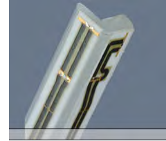
Figure 4-1 E-field Free-space Probe
