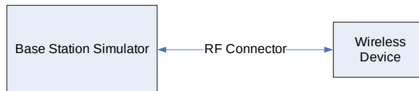
Figure 1-2 Power Measurement Setup
