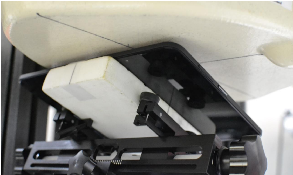
Test Setup Photo 8 – Read, Back Side, North Antenna at 5 mm
