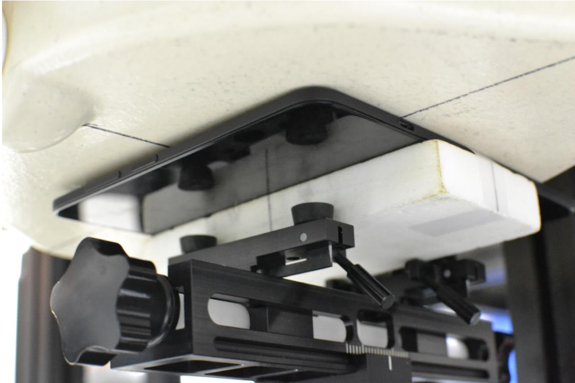
Test Setup Photo 7 – Read, Back Side, South Antenna at 5 mm
