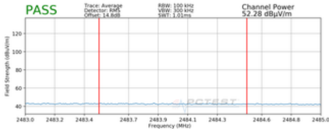
Plot 7-251. Radiated Restricted Upper Band Edge Measurement SISO SOUTH (Average)
