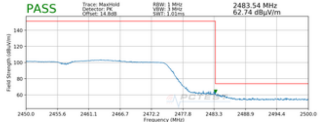
Plot 7-282. Radiated Restricted Upper Band Edge Measurement SISO NORTH (Peak)
