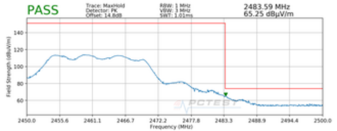
Plot 7-292. Radiated Restricted Upper Band Edge Measurement MIMO (Peak)
