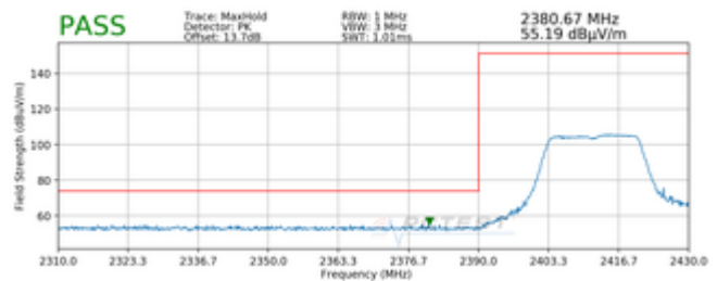
Plot 7-256. Radiated Restricted Lower Band Edge Measurement SISO NORTH (Peak)
