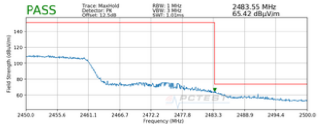
Plot 7-246. Radiated Restricted Upper Band Edge Measurement SISO SOUTH (Peak)
