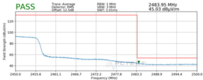
Plot 7-273. Radiated Restricted Upper Band Edge Measurement SISO NORTH (Average)
