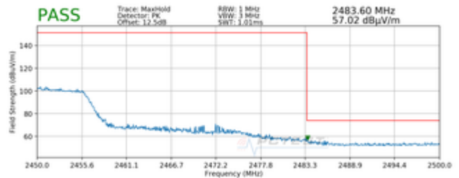
Plot 7-274. Radiated Restricted Upper Band Edge Measurement SISO NORTH (Peak)
