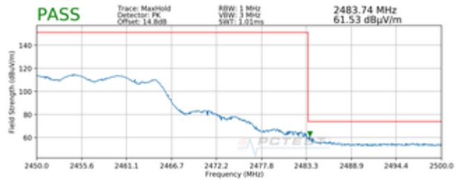
Plot 7-290. Radiated Restricted Upper Band Edge Measurement MIMO (Peak)
