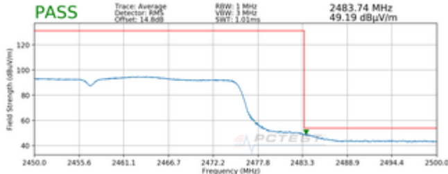
Plot 7-281. Radiated Restricted Upper Band Edge Measurement SISO NORTH (Average)
