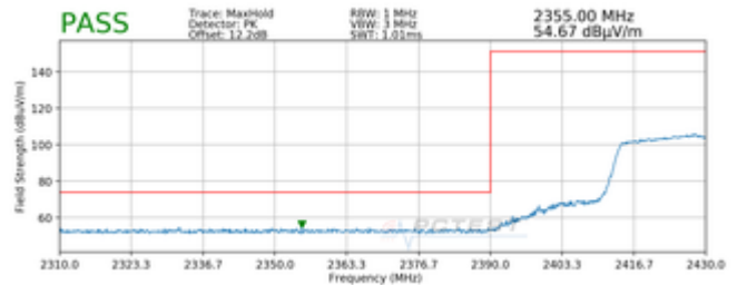
Plot 7-272. Radiated Restricted Upper Band Edge Measurement SISO NORTH (Peak)
