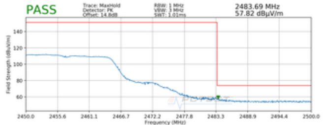
Plot 7-230. Radiated Restricted Upper Band Edge Measurement SISO SOUTH (Peak)
