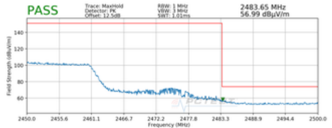
Plot 7-276. Radiated Restricted Upper Band Edge Measurement SISO NORTH (Peak)
