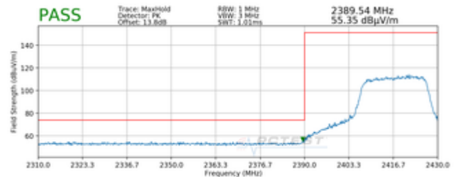
Plot 7-228. Radiated Restricted Upper Band Edge Measurement SISO SOUTH (Peak)
