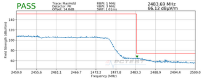
Plot 7-252. Radiated Restricted Upper Band Edge Measurement SISO SOUTH (Peak)
