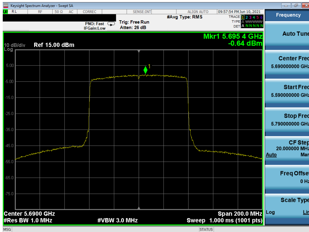
Plot 7-263. Power Spectral Density Plot SISO NORTH (80MHz BW 802.11ax (UNII Band 2C) – Ch. 138)
