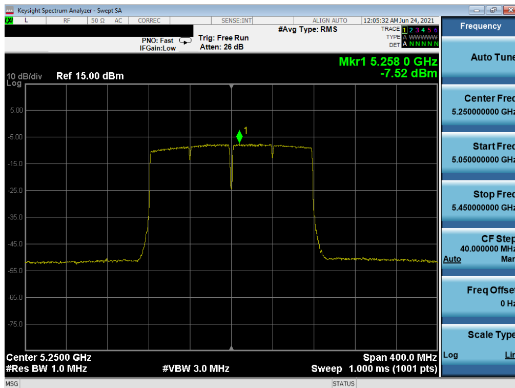
Plot 7-351. Power Spectral Density Plot MIMO NORTH (160MHz BW 802.11ac (UNII Band 1/2A) – Ch. 50)
