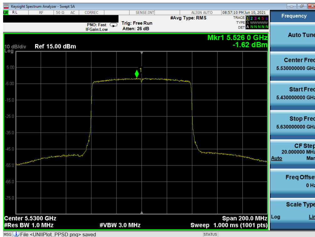
Plot 7-191. Power Spectral Density Plot SISO SOUTH (80MHz BW 802.11ax (UNII Band 2C) – Ch. 106)
