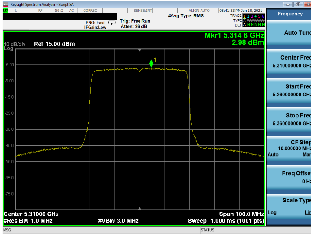
Plot 7-170. Power Spectral Density Plot SISO SOUTH (40MHz BW 802.11ax(UNII Band 2A) – Ch. 62)
