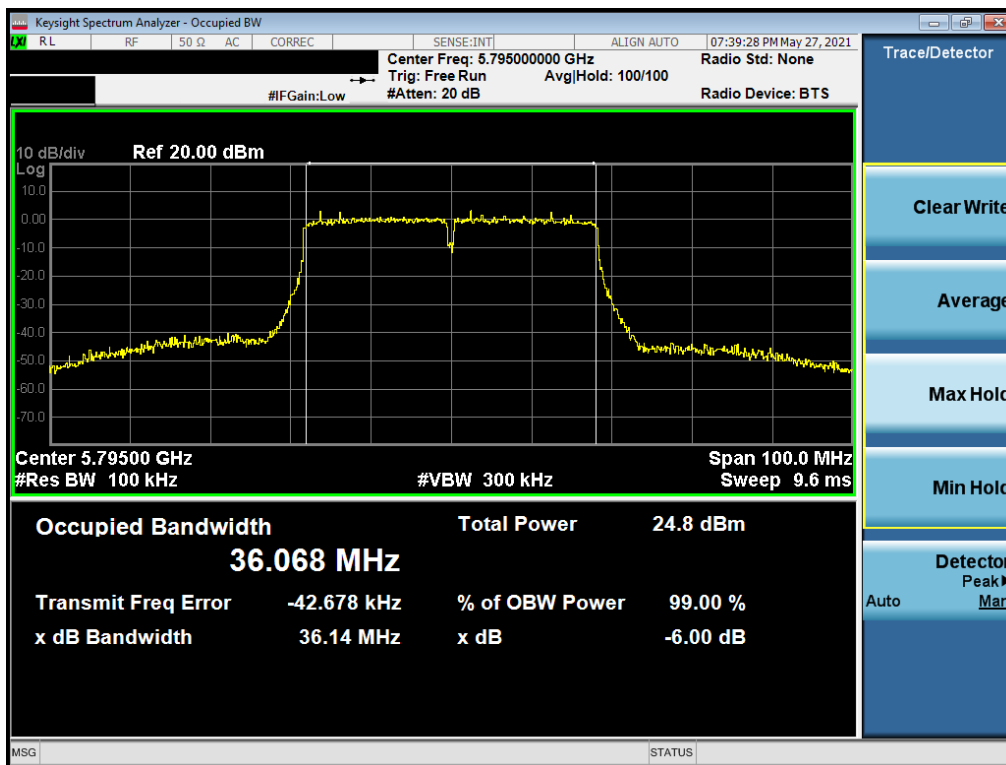
Plot 7-136. 6dB Bandwidth Plot SISO NORTH (40MHz BW 802.11n (UNII Band 3) – Ch. 159)
