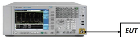
Figure 7-4. Test Instrument & Measurement Setup
