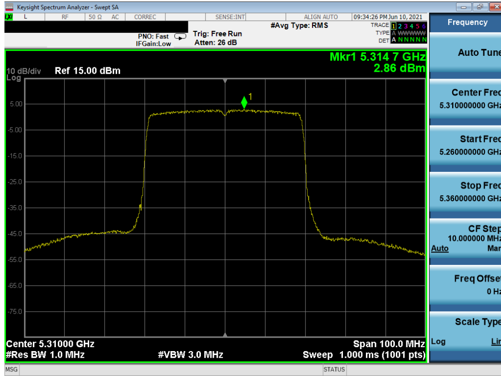
Plot 7-240. Power Spectral Density Plot SISO NORTH (40MHz BW 802.11ax (UNII Band 2A) – Ch. 62)
