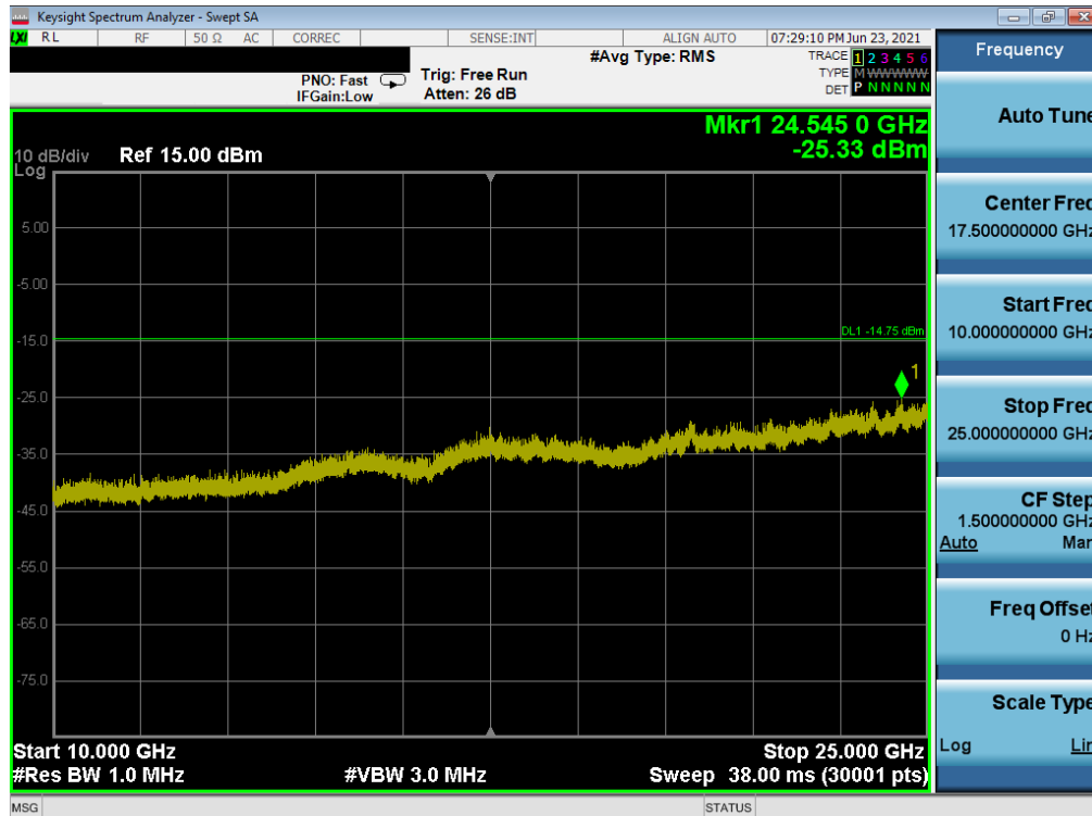
Plot 7-74. Conducted Spurious Plot (Bluetooth, 1Mbps – Ch. 0) – North Antenna
