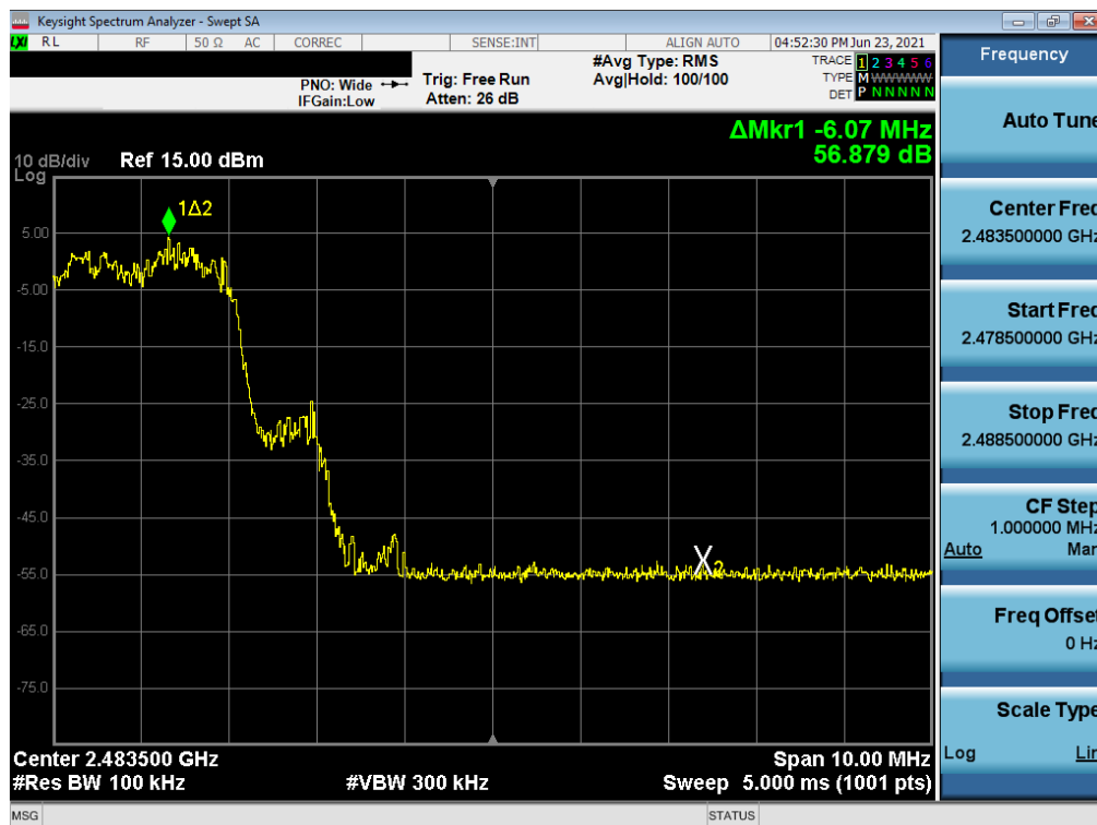
Plot 7-58. Band Edge Plot (Bluetooth with Hopping Enabled, 3 Mbps) – South Antenna
