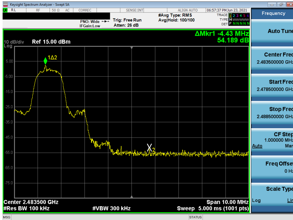
Plot 7-60. Band Edge Plot (Bluetooth with Hopping Disabled, 3 Mbps – Ch. 78) – North Antenna
