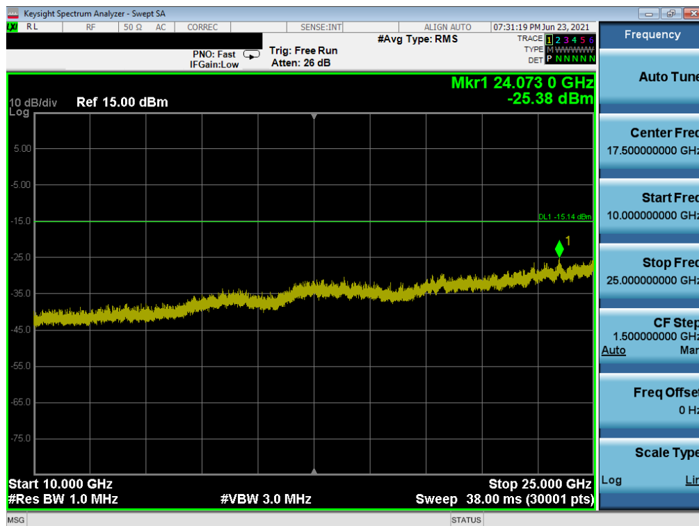
Plot 7-76. Conducted Spurious Plot (Bluetooth, 1Mbps – Ch. 39) – North Antenna
