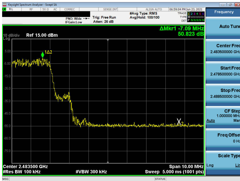
Plot 7-62. Band Edge Plot (Bluetooth with Hopping Enabled, 3 Mbps) – North Antenna
