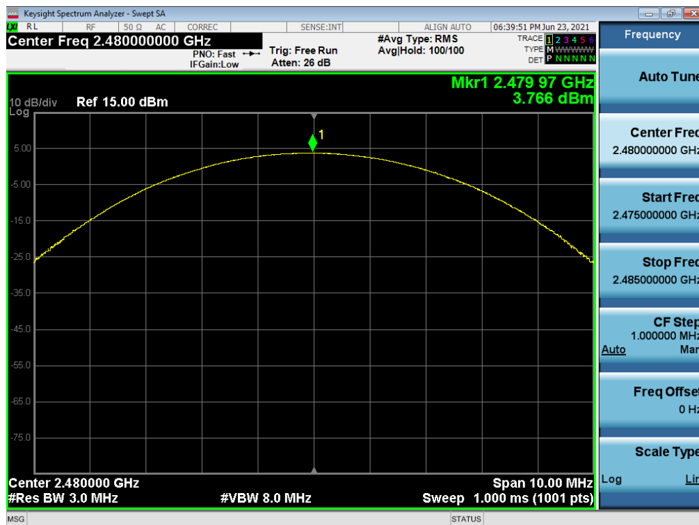
Plot 7-45. Peak Conducted Power (3Mbps – Ch. 78) – North Antenna
