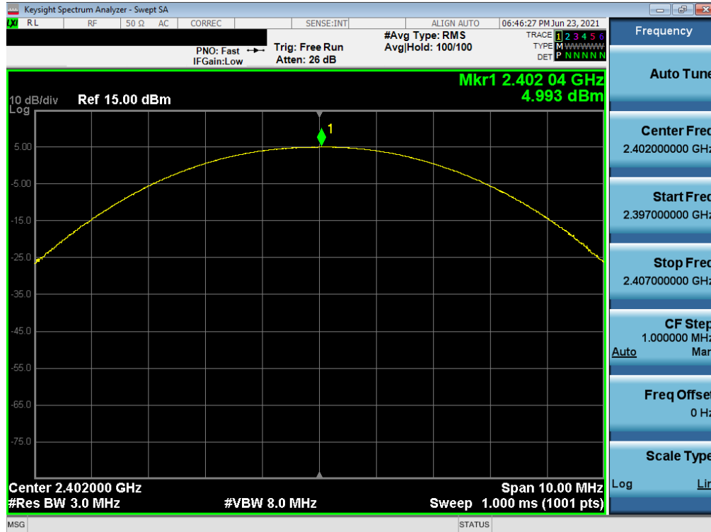
Plot 7-40. Peak Conducted Power (2Mbps – Ch. 0) – North Antenna
