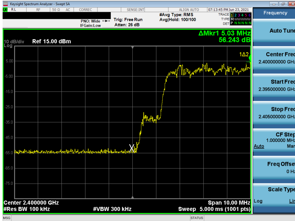
Plot 7-61. Band Edge Plot (Bluetooth with Hopping Enabled, 3 Mbps) – North Antenna
