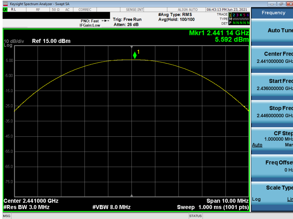
Plot 7-38. Peak Conducted Power (1Mbps – Ch. 39) – North Antenna
