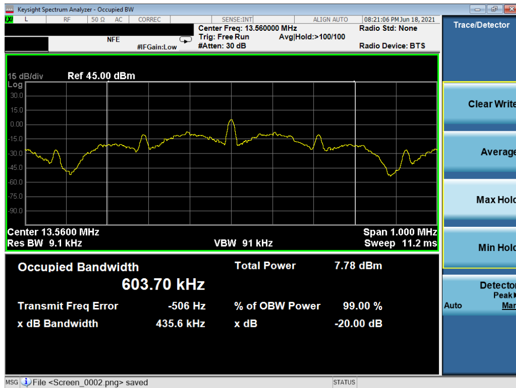
Figure 7-2. Occupied Bandwidth Plot
