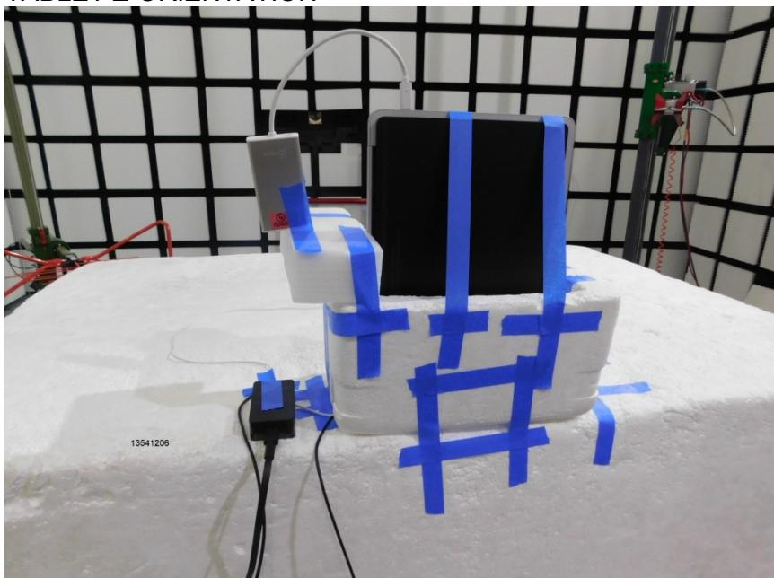
**AC MAINS LINE CONDUCTED MEASUREMENT SETUP**
