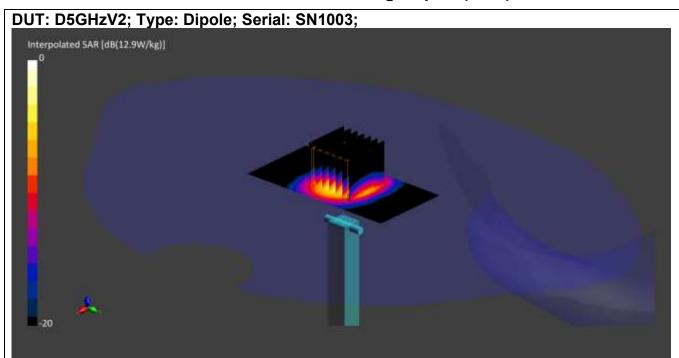
Communication System: CW UID: 0; Frequency: 5600.0 MHz; Duty Cycle: 1; Medium: HSL; Site65\_17Feb2021\_110903\_Head - 3500 5250 5600 5750 5%; Medium parameters used: f = 5600.0 MHz;  $\sigma$  = 5.2 S/m;  $\epsilon_r$  = 35.7;  $\rho$  = 1000 kg/m3;  $\Delta\epsilon_r$  = 0.50 %;  $\Delta\sigma$  = 2.66 %; No correction
