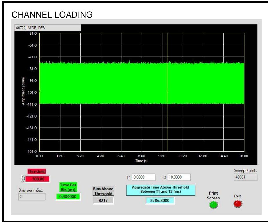
The level of traffic loading on the channel by the EUT is 32.87%
