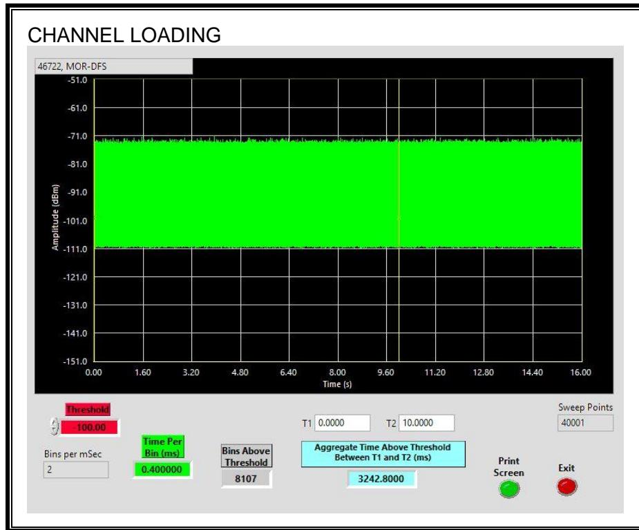
The level of traffic loading on the channel by the EUT is 32.43%
