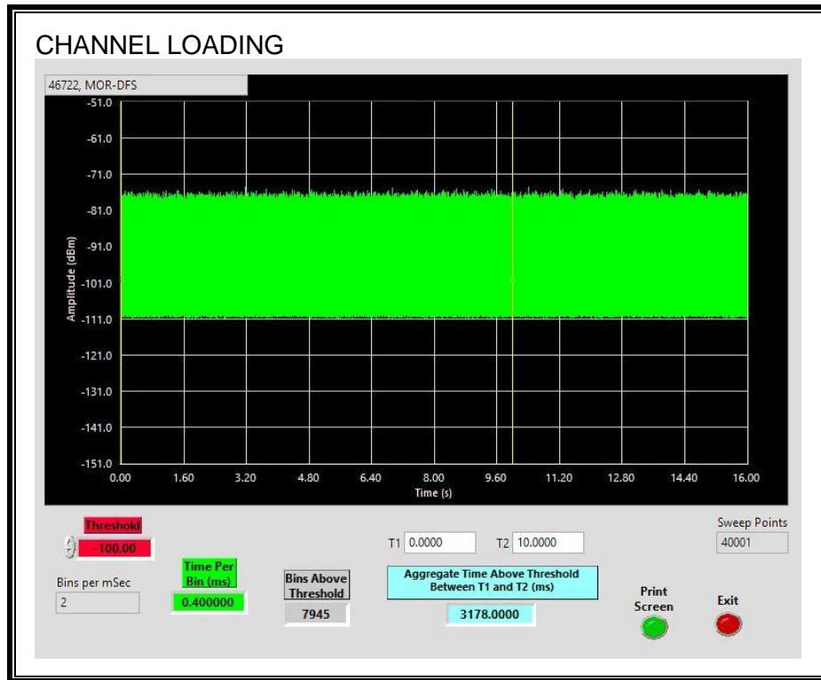
The level of traffic loading on the channel by the EUT is 31.78%
