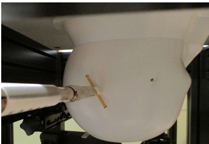
2.4 GHz Dipole Placed at Location A in 90° Orientation (10mm Spacer)
