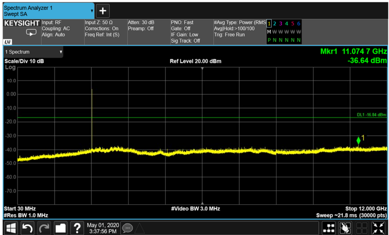
Figure 9-18 Conducted Spurious Emissions 30-12000 MHz (Ch. 19)
