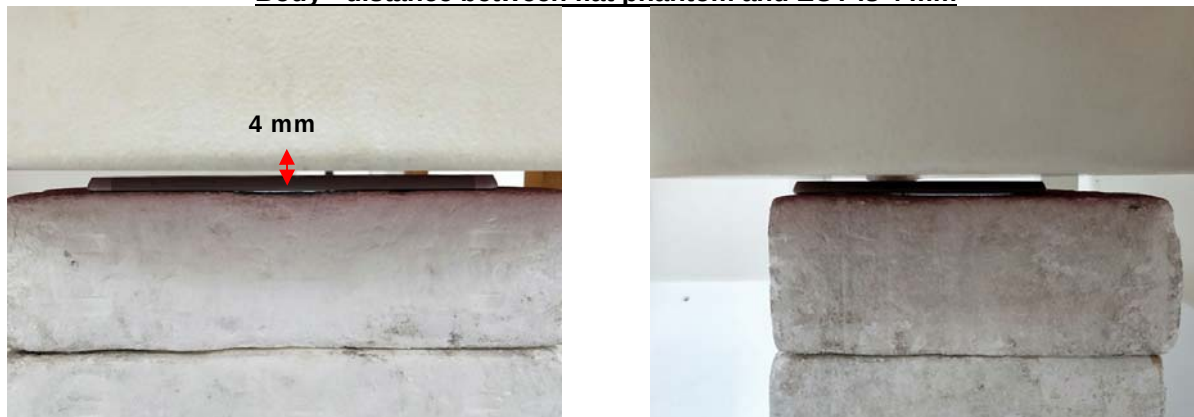
Fig.8 EUT Back side to flat phantom
