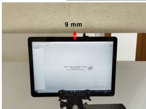
Fig.11 EUT Top side to flat phantom
