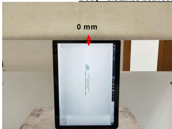
Fig.6 EUT Right side to flat phantom
