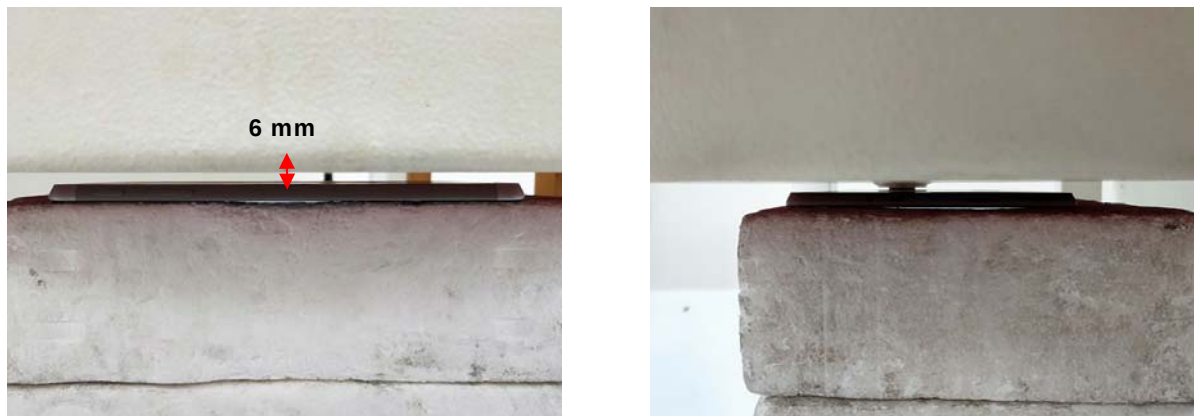
Fig.10 EUT Back side to flat phantom
