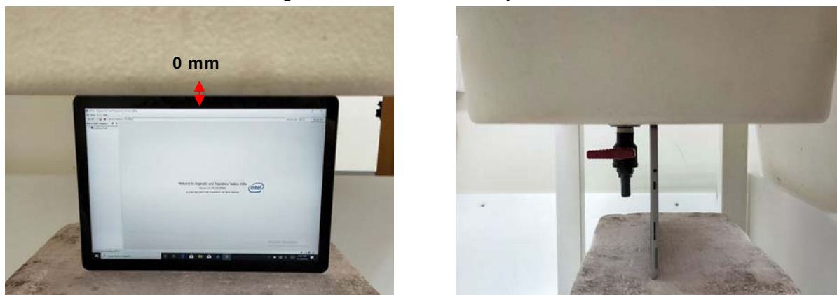
Fig.4 EUT Top side to flat phantom
