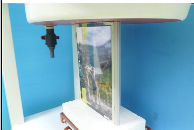
Body - Right Side of EUT at 0 mm w/ Keyboard
