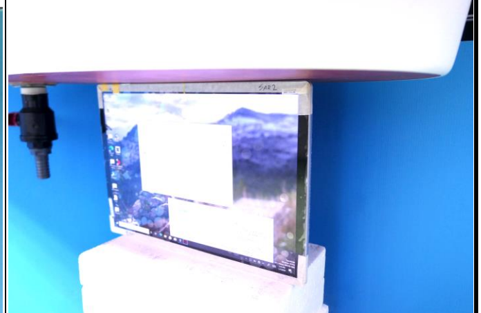
Body - Top Side of EUT at 0 mm w/o Keyboard
