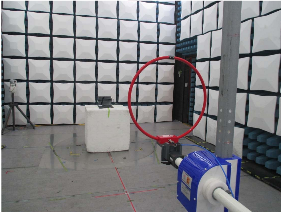
Figure 1 Radiated Spurious Emissions Test Setup (9k-30MHz)
