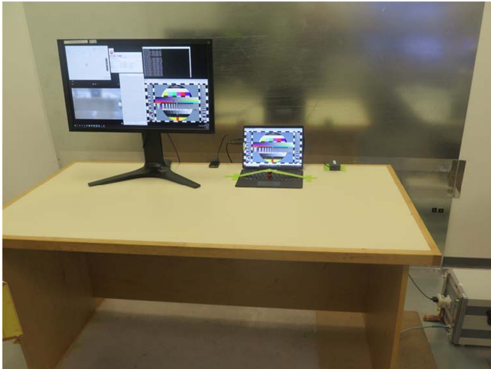
Figure 3 AC Line Conducted Emissions
