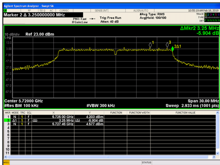
Plot 9-143. 6-dB Bandwidth Chain 0 802.11a (Ch. 144)
