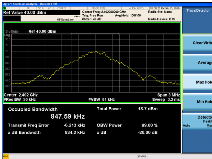
Figure 9-4 20dB Bandwidth (Ch. 0, 1-DH5)
