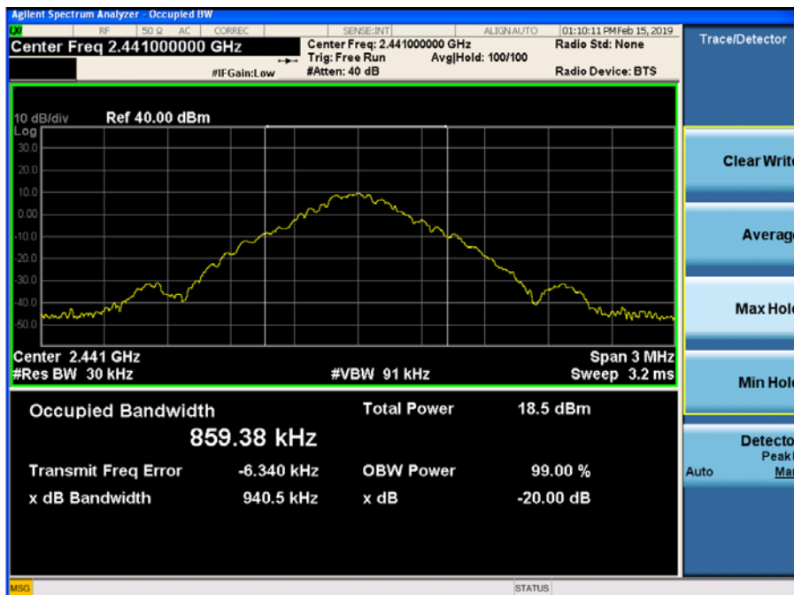
Figure 9-5 20dB Bandwidth (Ch. 39, 1-DH5)
