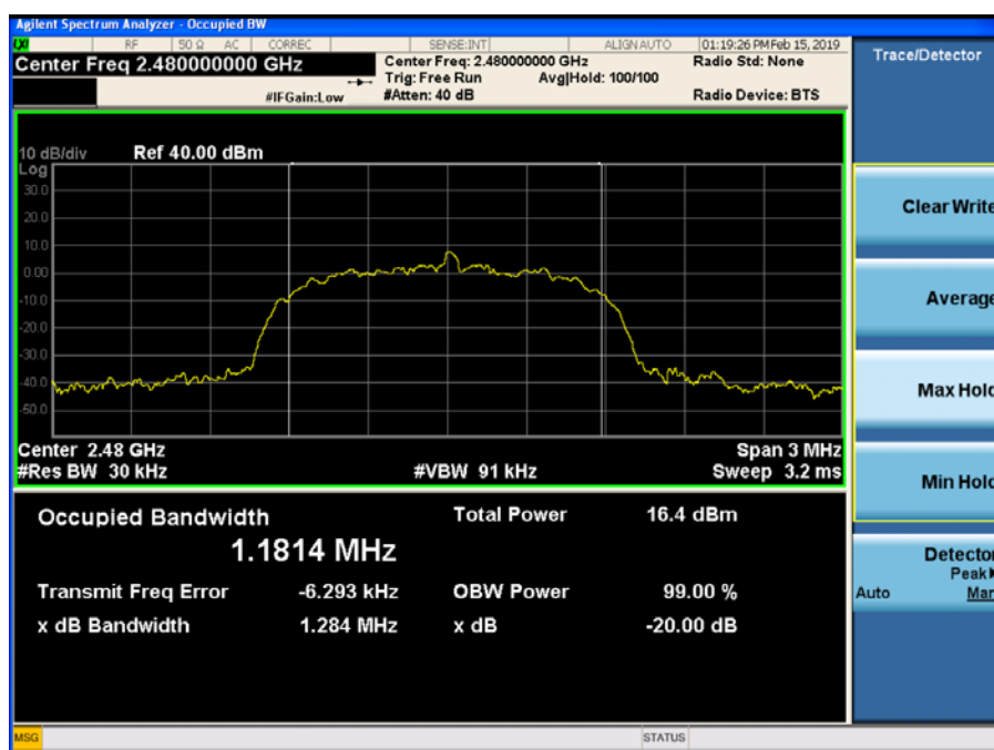
Figure 9-12 20dB Bandwidth (Ch. 78, 3-DH5)
