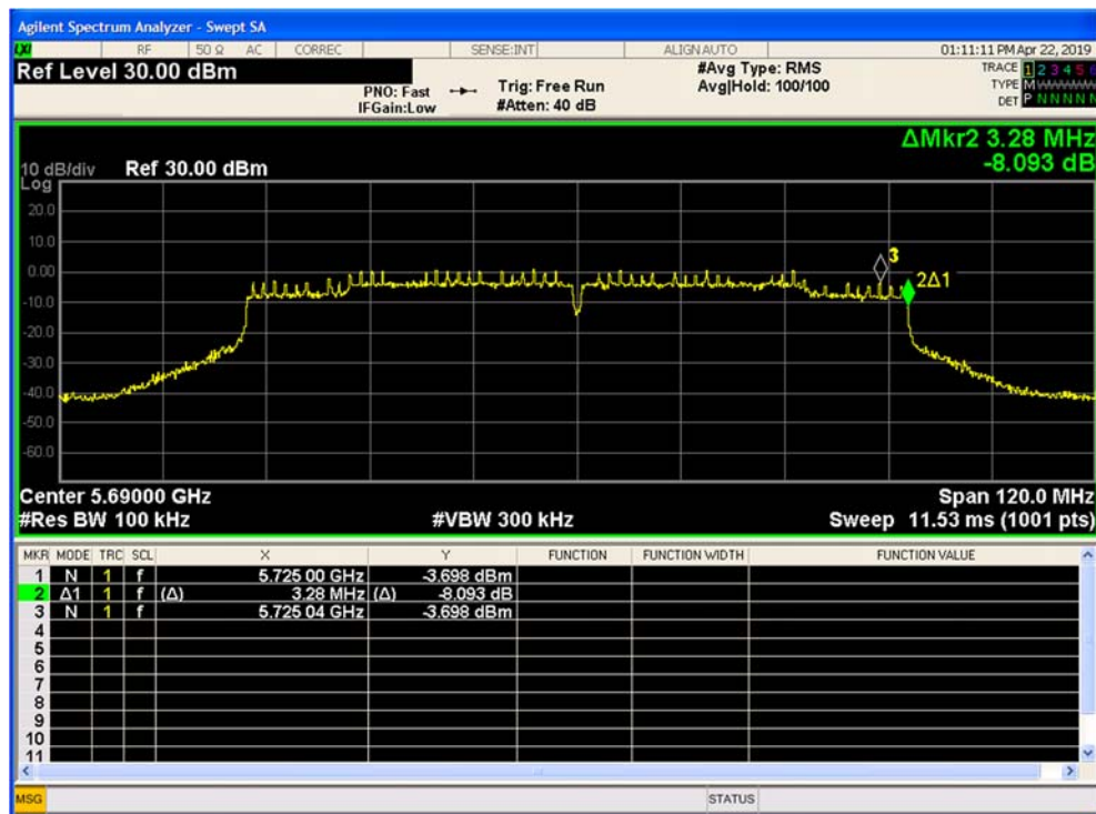
Figure 9-170. 6-dB Bandwidth SISO Chain B 802.11ac VHT80 (Ch. 138)
