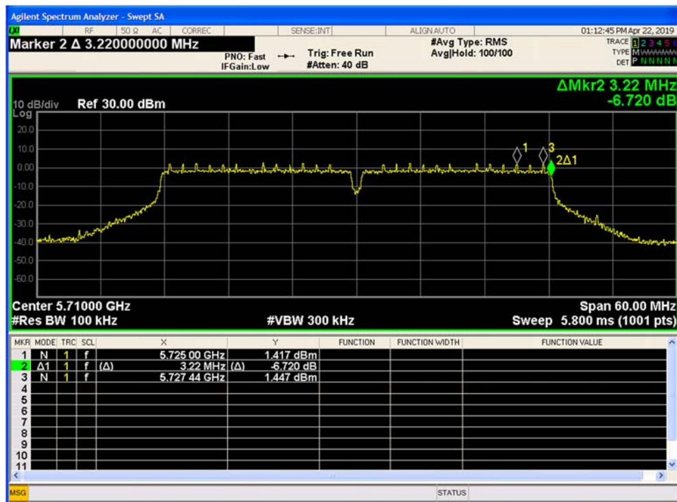
Figure 9-162. 6-dB Bandwidth SISO Chain B 802.11ac VHT40 (Ch. 142)
