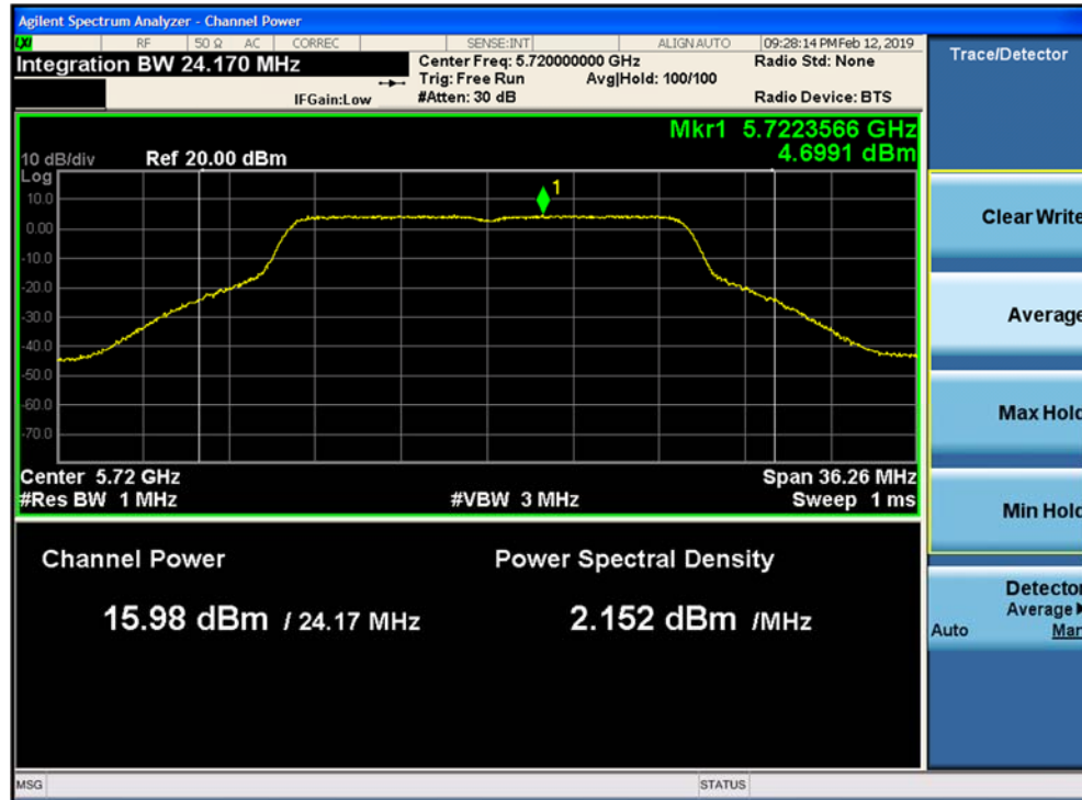
Figure 9-179 Maximum Conducted Output Power and PSD SISO Chain A 802.11a (Ch. 144)
