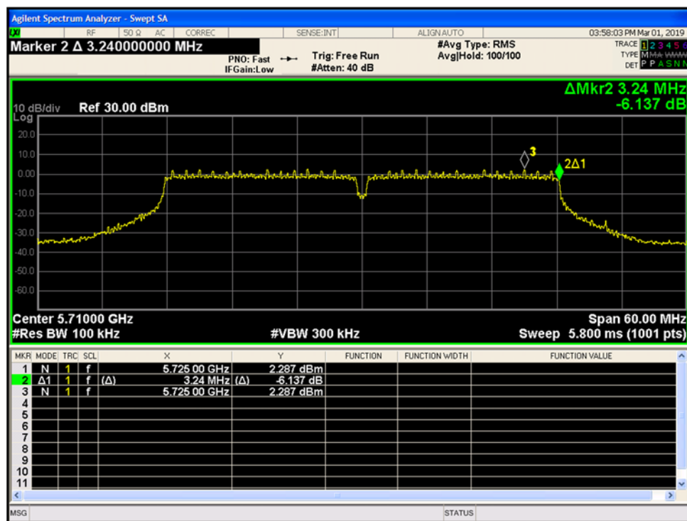
Figure 9-166. 6-dB Bandwidth Chain B 802.11ac VHT40 (Ch. 142)
