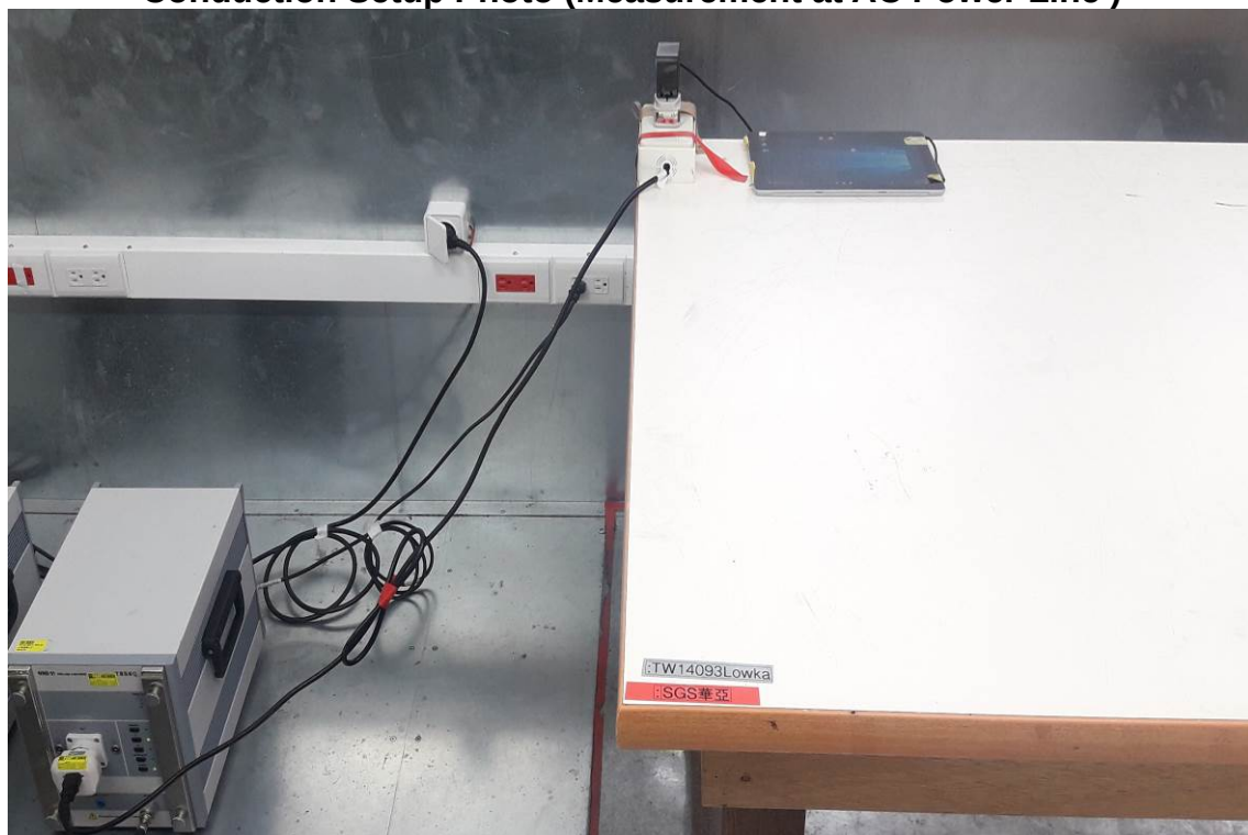
Conduction Setup Photo (Measurement at AC Power Line )
