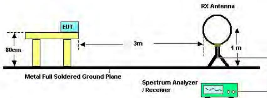
For Radiated Emissions: 30MHz~1GHz
