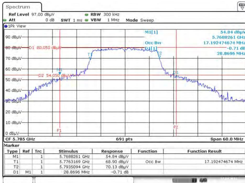
**26dB Bandwidth and 99% Occupied Bandwidth Plot on Configuration IEEE 802.11a / Chain 2 / 5825 MHz**
