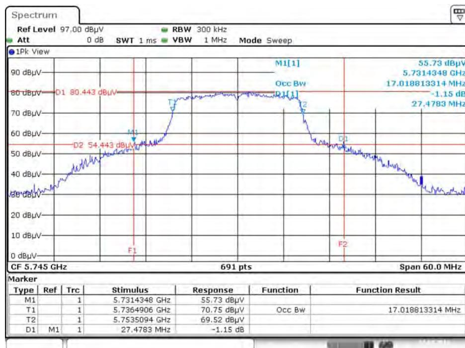
**26dB Bandwidth and 99% Occupied Bandwidth Plot on Configuration IEEE 802.11a / Chain 2 / 5785 MHz**
