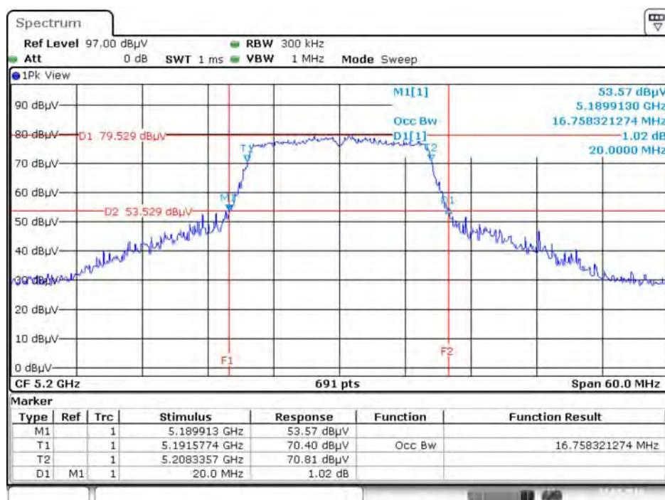
**26dB Bandwidth and 99% Occupied Bandwidth Plot on Configuration IEEE 802.11a / Chain 2 / 5240 MHz**
