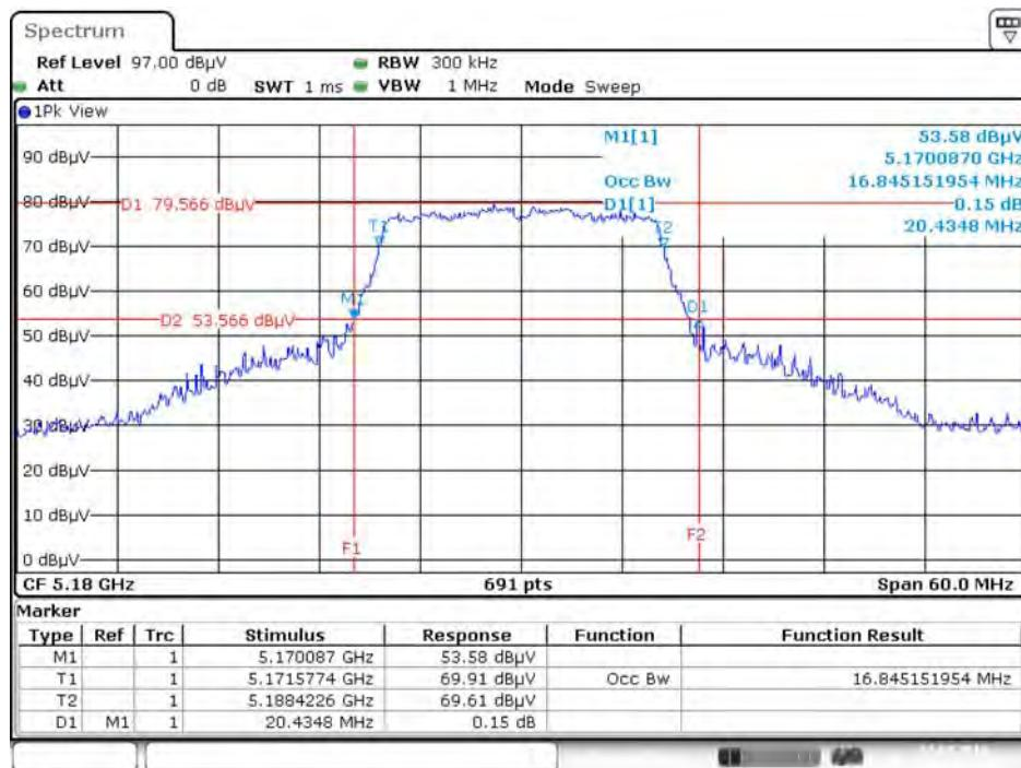
**26dB Bandwidth and 99% Occupied Bandwidth Plot on Configuration IEEE 802.11a / Chain 2 / 5200 MHz**
