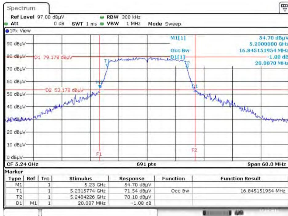
**26dB Bandwidth and 99% Occupied Bandwidth Plot on Configuration IEEE 802.11a / Chain 2 / 5745 MHz**
