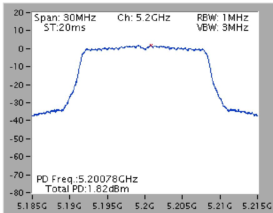
Power Density Plot on Configuration IEEE 802.11a / Chain 2 / 5745 MHz
