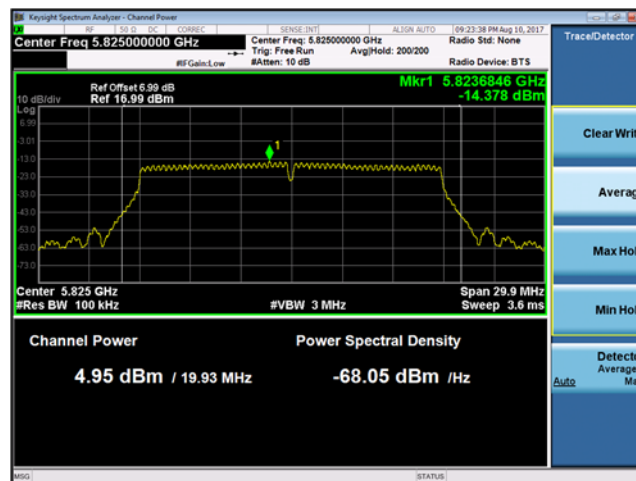
Plot 9-18. Maximum Power Spectral Density 802.11n (Ch. 165)
