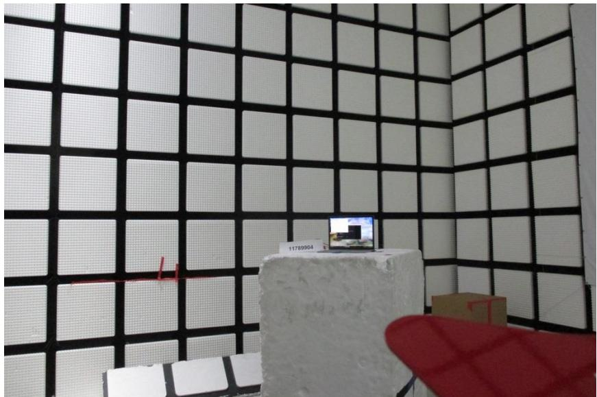
**POWERLINE CONDUCTED EMISSIONS MEASUREMENT SETUP**
