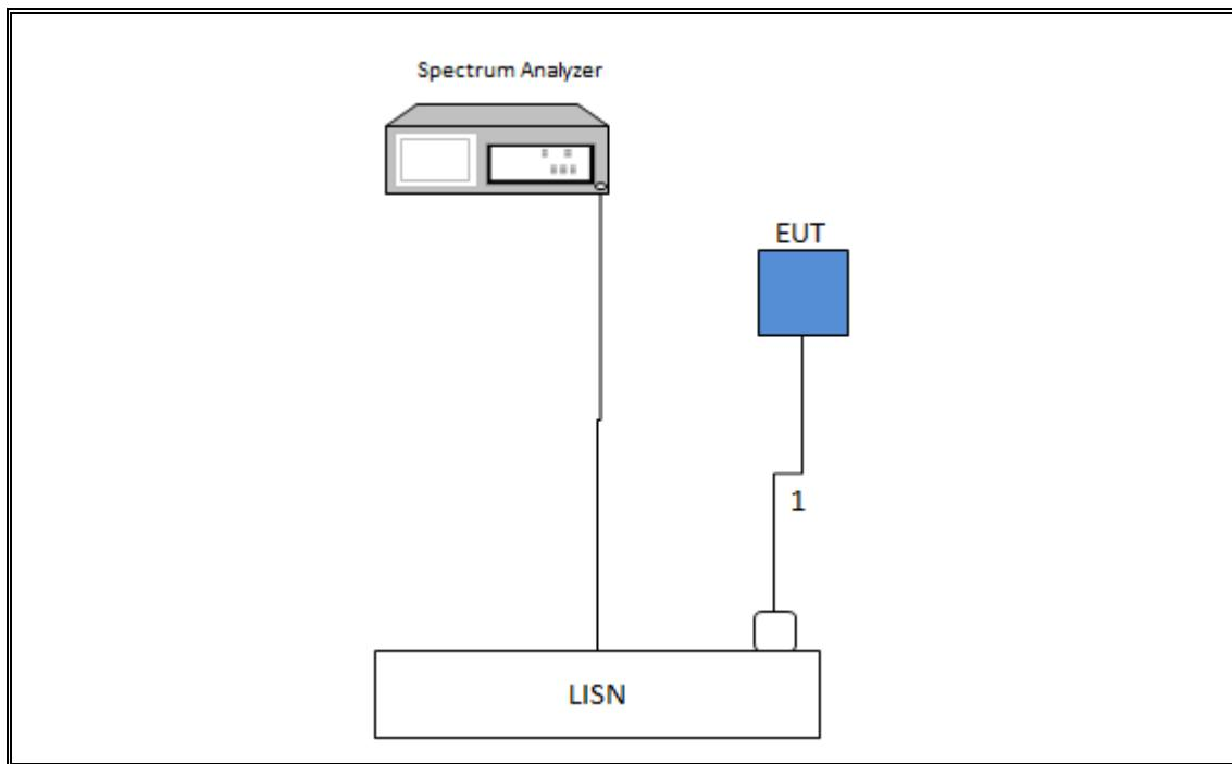
**TEST SETUP- AC LINE CONDUCTED: LAPTOP CONFIGURATION**
