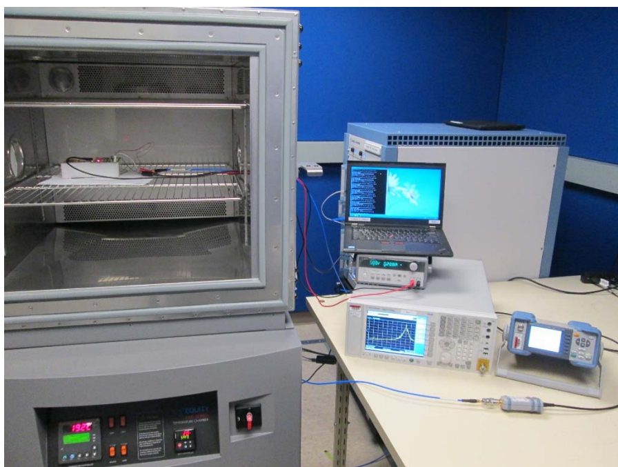
Fig.6 Antenna port Conducted Measurements Test Setup
