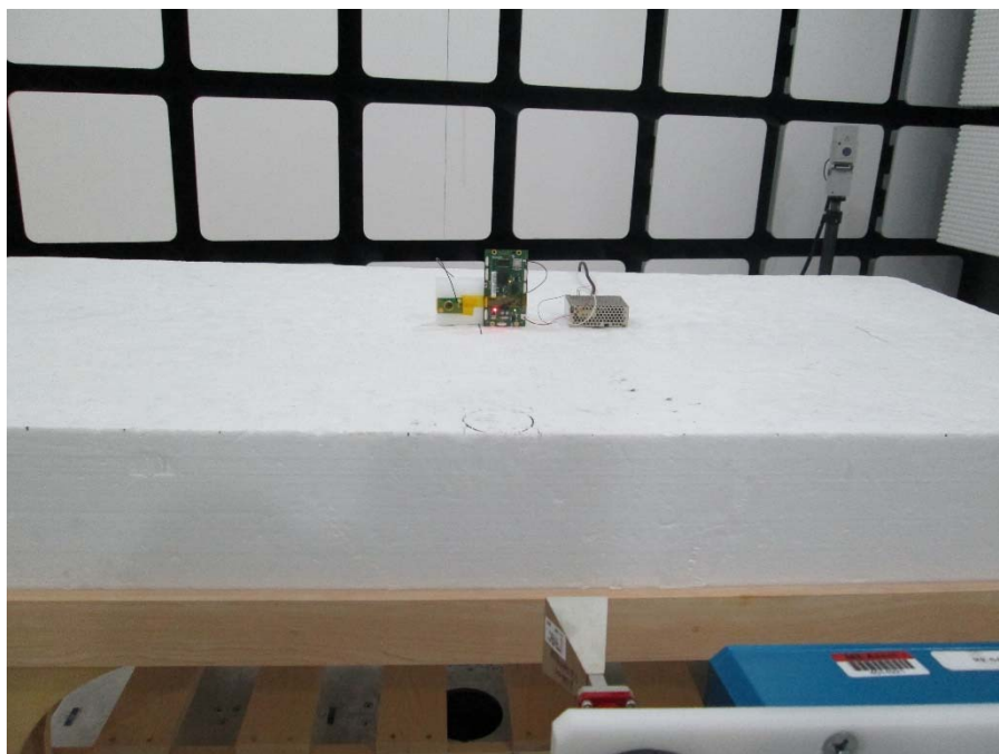
Fig.5 Radiated Emissions Test Setup (18GHz – 26.5 GHz)
