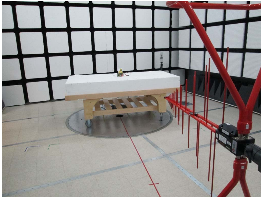
Fig.3 Radiated Emissions Test Setup (30MHz – 1GHz)
