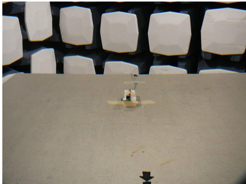
**1.5 Radiated Emission below 1GHz Rear View @ 3 Meter**
