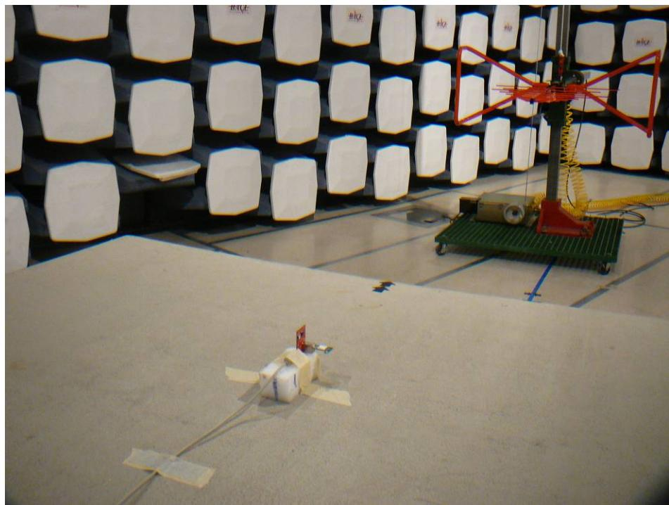
**1.6 Radiated Emission above 1 GHz Rear View @ 3 Meter**
