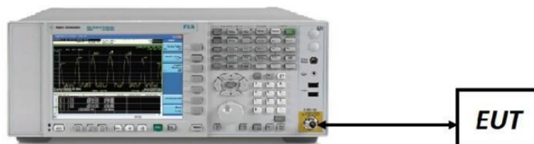
Figure 7-4. Conducted Test Setup for Band Edge > 1GHz
