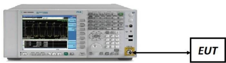
Figure 7-4. Conducted Test Setup for Band Edge > 1GHz
