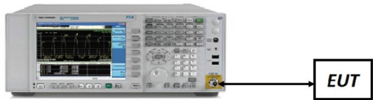
Figure 7-4. Conducted Test Setup > 1GHz
