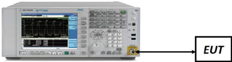
Figure 7-4. Conducted Test Setup > 1GHz
