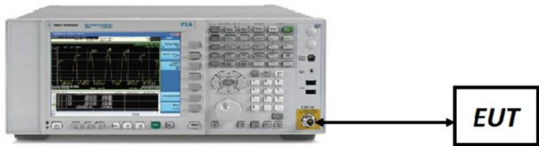
Figure 7-4. Conducted Test Setup > 1GHz
