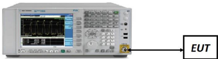
Figure 7-4. Conducted Test Setup > 1GHz
