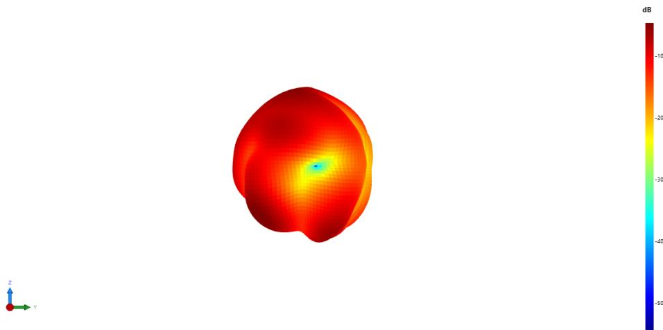
Max Antenna 3D Radiation Pattern 5150-5250 MHz
