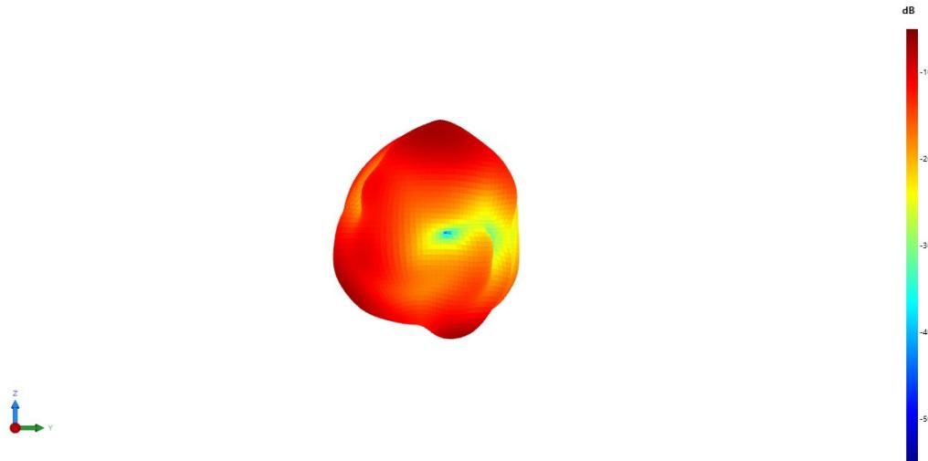
Max Antenna 3D Radiation Pattern 5150-5250 MHz
