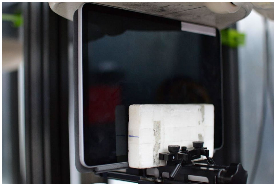
Test Setup Photo 4 – Body, Top Edge at 0mm with keyboard, Antenna R and L
