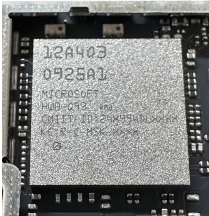
Figure 3: Wifi BT Module (Model no. HWB-Q93)
