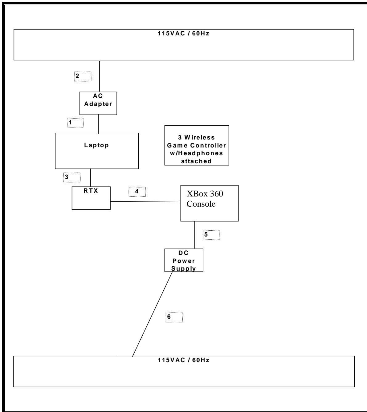
SETUP DIAGRAM FOR TESTS, CONFIGURATION 2
