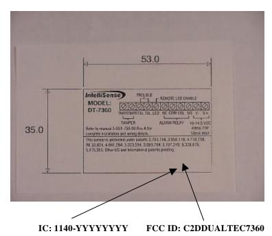
Hook-up/FCC/IC Label above will be located on the inside front cover
