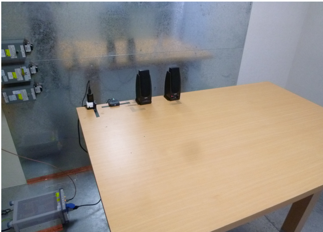
Photograph 6: Set-up for for Mains Conducted testing Front
