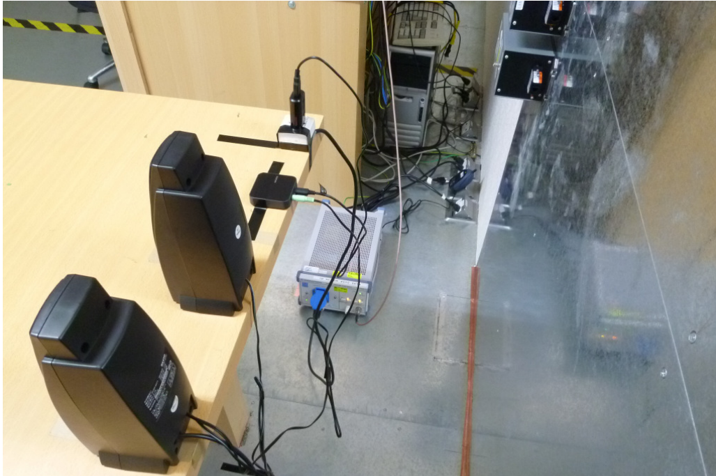
Photograph 5: Set-up for for Mains Conducted testing Back
