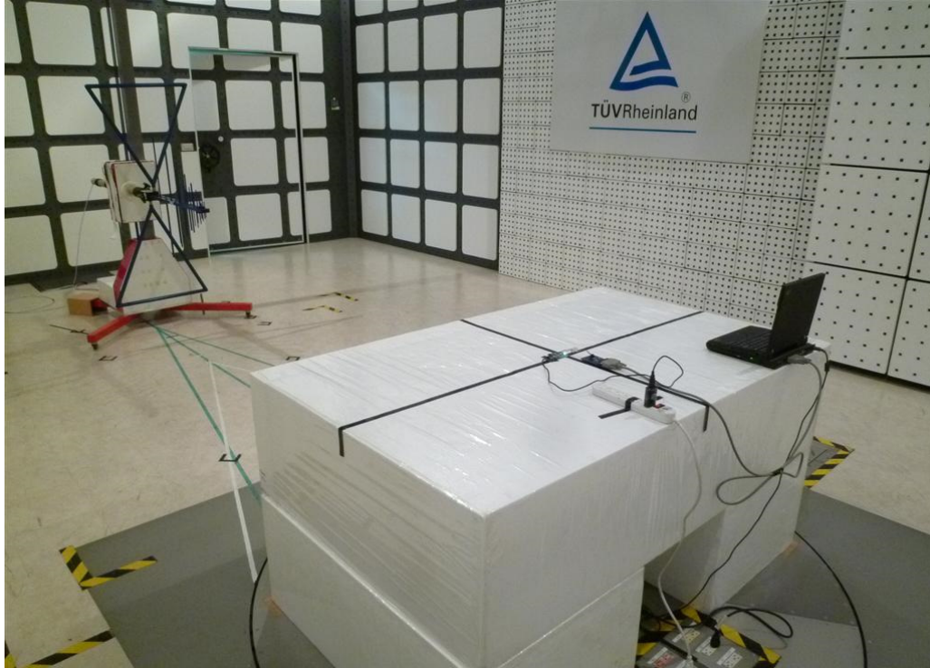
Photograph 2: Set-up for Spurious Emissions (Back View 1)
