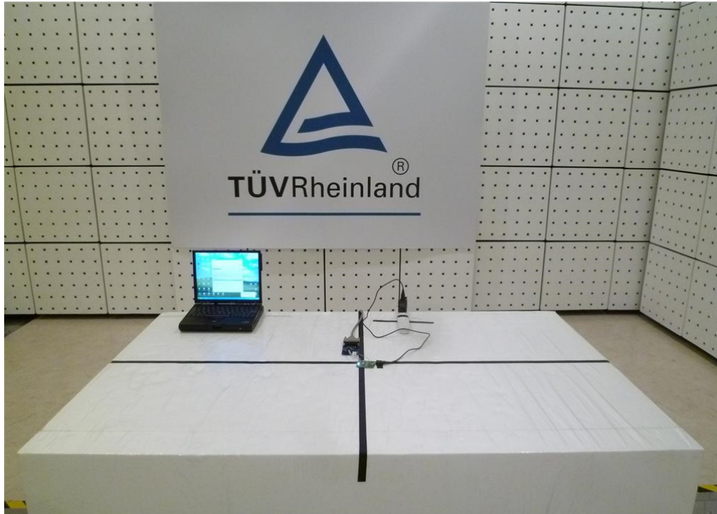
Photograph 1: Set-up for Spurious Emissions (Front View)
